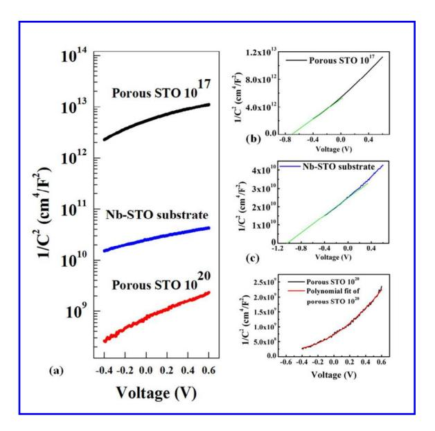
Figure 4:  $1/C^2$  vs. V plots of various samples measured at 1 kHz with an amplitude of 10 mV. (a) The results for the three samples studied - porous STO  $10^{20}$ , Nb-STO substrate and porous STO  $10^{17}$  shown together in logarithmic scale, (b) and (c) Mott-Schottky linear fits of the results for porous STO  $10^{17}$  and Nb-doped substrate, respectively and (d) polynomial fit of the results for porous STO  $10^{20}$ .
