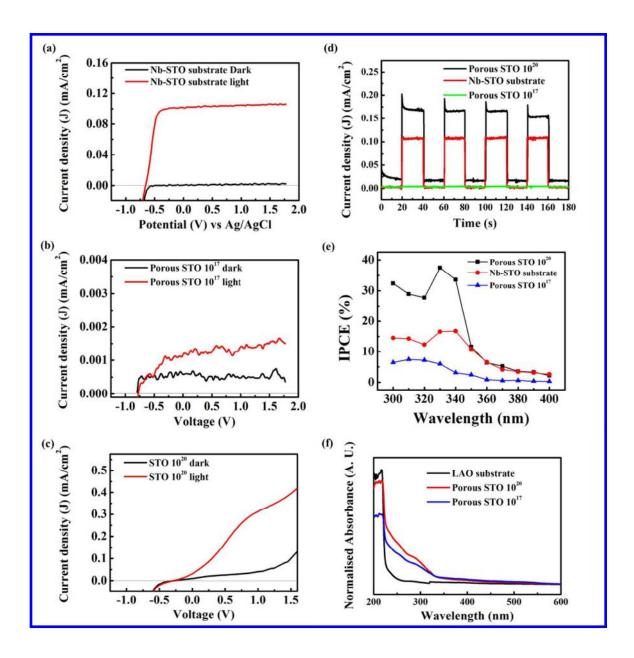
Figure 3: J-V characteristics of (a) Nb-STO substrate, (b) porous STO 10<sup>17</sup> and (c) porous STO 10<sup>20</sup>. (d) Chronoamperometry results of the samples. The potential used was 0.5 V vs. the Ag/AgCl (3M KCl) electrode for Chronoamperometry results. (e) Incident Photon to Current Efficiency (IPCE) results measured at 0.3 V vs. Ag/AgCl and (f) UV-Vis absorption spectra.
