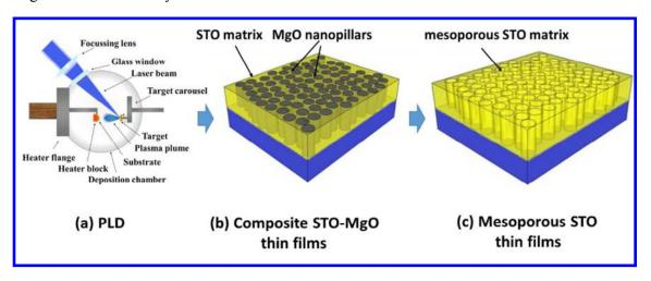
Figure 1: Schematic diagram showing (a) the PLD setup, (b) the PLD-grown columnar composite thin film containing STO matrix and MgO nanopillars and (c) the mesoporous STO thin film, after etching out the MgO nanopillars
