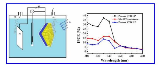
Very high surface area mesoporous thin films grown by pulsed laser deposition (PLD) for photoelectrochemical water splitting
