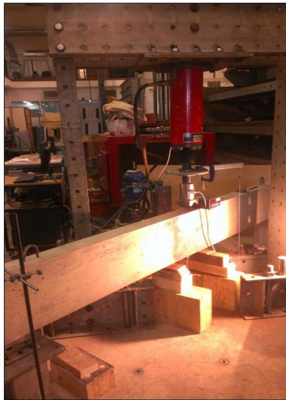
Figure 7 Photo of large beam in test rig
