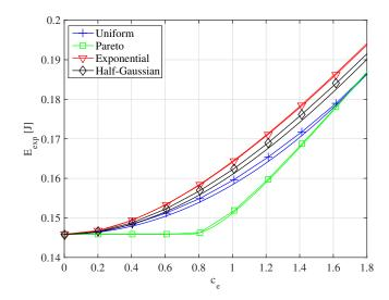
Figure 3. Average energy consumption  $E_{\rm exp}$  vs.  $c_{\rm e}$ . The average query volume was set to r = 81,920 b. For the case of Pareto distribution, we used  $\alpha_{\rm e} = 4$ . Lines with markers: Monte Carlo experiments; Lines without markers: theoretical predictions.
