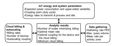
Figure 2. Conceptual illustration of the linkage between: IoT system parameters, cloud billing & autoscaling, and data gathering. When parameters from two out of three domains are provided, our analytic framework can be used to tune the parameters of the third.
