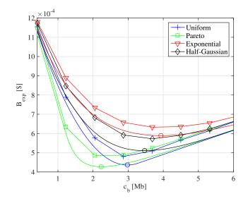
Figure 5. Average billing cost  $B_{\rm exp}$  vs.  $c_{\rm b}$ . The average query volume per device was set to r = 163,840 b and the experiment corresponds to n = 10 devices. For the case of Pareto distribution, we used  $\alpha_{\rm e} = 4$ . Lines with markers: Monte Carlo experiments; Lines without markers: theoretical predictions. The circles indicate minimum billing values as predicted by the analysis in Section III.
