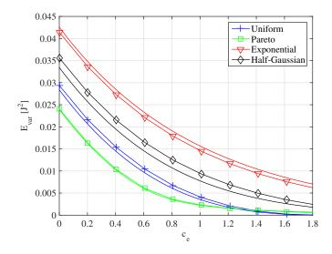
Figure 4. One-sided energy consumption  $E_{\rm var}$  vs.  $c_{\rm e}$ . The average query volume was set to r = 81,920 b. For the case of Pareto distribution, we used  $\alpha_{\rm e} = 4$ . Lines with markers: Monte Carlo experiments; Lines without markers: theoretical predictions.
