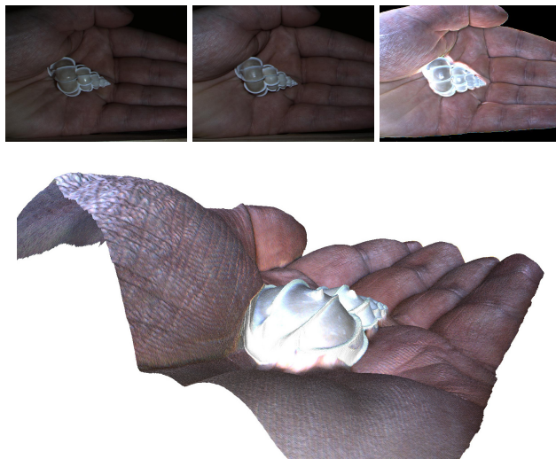
Figure 1. The first row shows two samples of near field images acquired under different lighting and different exposure (both unknown) and the computed albedo. Below it is the shape reconstructed using the proposed semi-calibrated PS approach.
