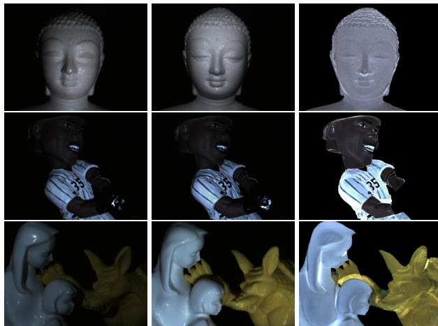
Figure 5. Darkest ( Left ) and brightest ( middle ) samples of our real datasets and the computed albedos ( Right ). Note that the coloring of the albedos is done by noting each pixel's position on the Bayer pattern of the raw data.
