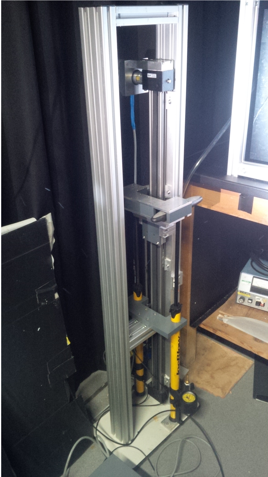
Plate 2: Photograph of the bike pump setup used to generate vortex rings within a stratified tank.
