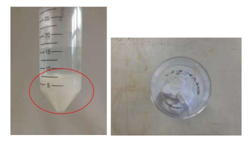
(a): Precipitates obtained from pH =8.75 after 30min bench reaction of SI.I
