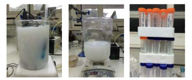
Figure 3. 4: A ttypical bench reaction when reactants addition in the first 10min (left); Bench reaction without reactants addition in the rest of 50min or 80min (middle); Free reaction after filtration for 1-3 days or a longer time (right);
