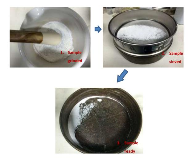
(c): The preparation of oxides for a reactivity test
