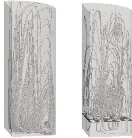
Figure 3: Cylinder without and with turbulence grid with streamlines at TDC for geometry 1 [8].
