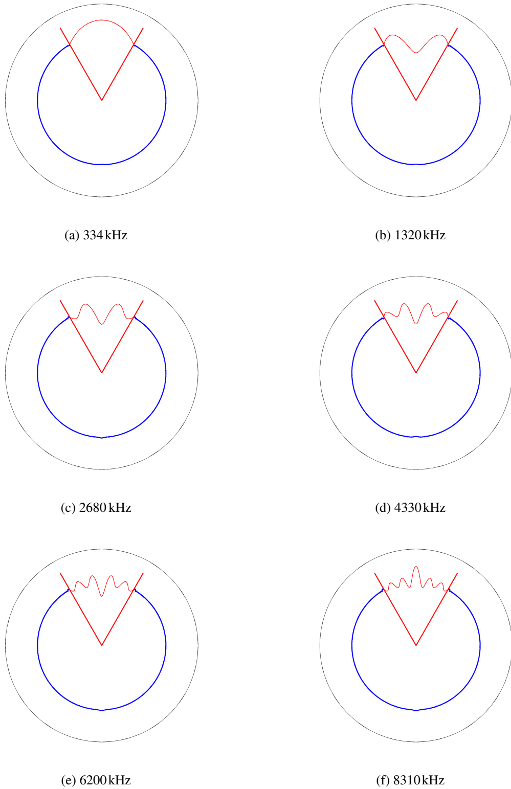
Figure 2.5: First six resonant mode shapes of the AMB. Blue marks the solid capsule and the red the bubble's free surface. The radial lines mark the edge of the cap at an angle \theta_0 = 0.52 from the axis of symmetry.
