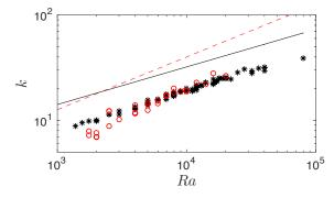
Figure 11: The predicted wavenumber from (5.1) (red dashed), together with data from direct numerical simulations (red circles) of three-dimensional convection (Hewitt *et al.* 2014). The corresponding prediction and results for two-dimensional convection, taken from Hewitt *et al.* (2013), are shown for comparison (black line and stars).
