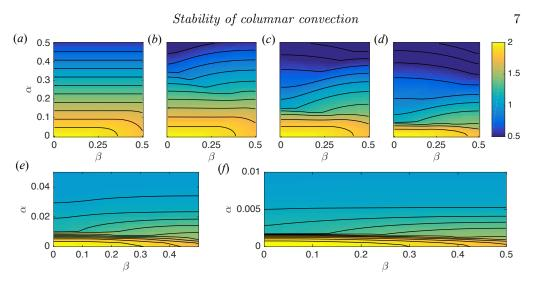
Figure 2: Density maps and contours of the maximum growth rate  $\operatorname{Re}\{\sigma_*\}$  maximized over  $\gamma$  for each value of  $(\alpha, \beta)$ , for a square base planform  $(\xi = 1)$  and different amplitudes: (a) A = 0, (b) A = 1, (c) A = 4, (d) A = 10, (e) A = 100, and (f) A = 500. The most unstable mode always has  $\alpha = \beta = \gamma = 0$ .
