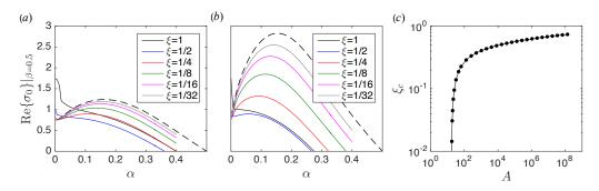
Figure 4: The maximum growth rate  $\operatorname{Re}\{\sigma_0\}$  at fixed  $\beta = 0.5$  and  $\gamma = 0$ , for different aspect ratios  $\xi$  of the base state as marked, and: (a)  $A = 2^5$ ; (b)  $A = 2^8$ . In each case, the dashed line shows the two-dimensional result (i.e. the limit  $\xi \to 0$ ). (c) The critical aspect ratio  $\xi_c$ , below which the columnar mode is the most unstable mode.
