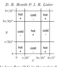
Figure 1: A schematic of the base flow (2.5) in the region  $0 \le x \le 2\pi/k^*$  and  $0 \le y \le 2\pi/(\xi k^*)$  in the (x, y) plane (shown here with  $\xi < 1$ ). The pattern periodically repeats outside this range. The temperature and the sign of the vertical velocity (w) in each rectangle is marked.
