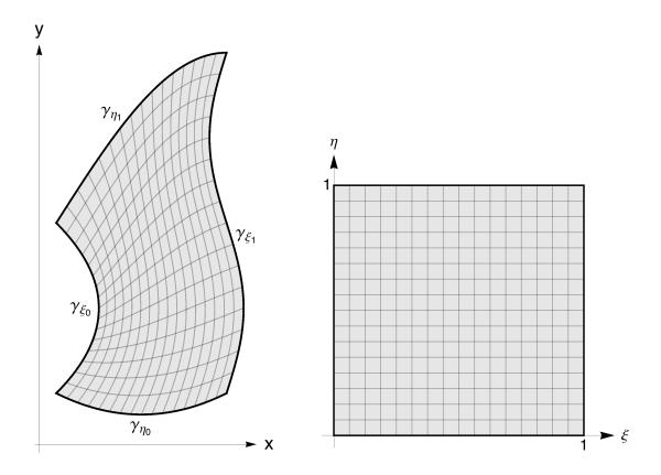
FIG. 3: Warped rectangle in physical space and logic space.
