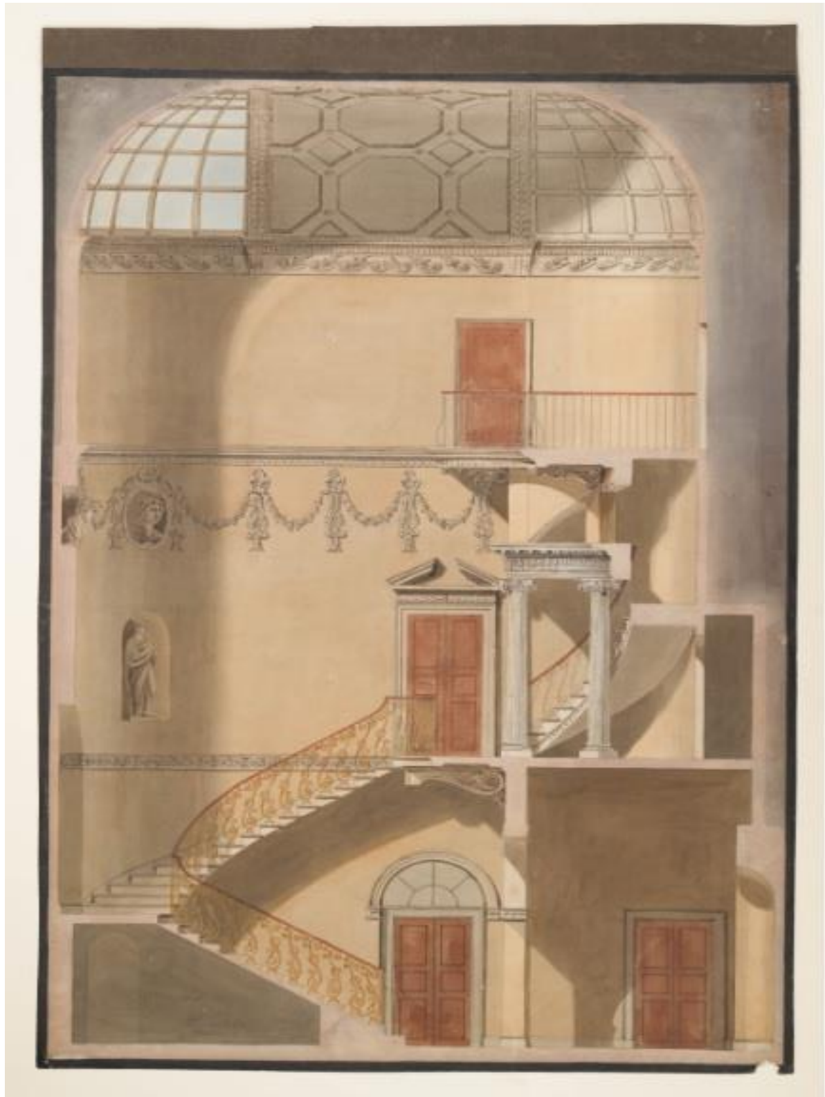
Fig. 5 Section of the staircase hall of No. 44 Berkeley Square, created for Sir John Soane's Royal Academy lectures on William Kent, 19th century.
