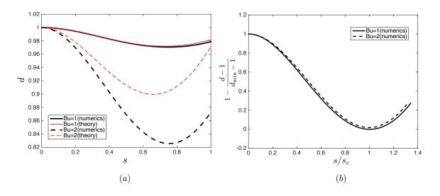
FIG. 13. (a) Comparison between the asymptotic solution for the deflection of the filaments (thin red lines) with the numerical solution (thick black lines) for Bu = 1 (solid) and Bu = 2 (dashed); (b) A closer look at the numerical solutions for Bu = 1 (solid) and Bu = 2 (dashed) indicated that up to a re-scaling they have the same shape ( $s_c$  is the value of the arclength at which the distance between the filaments is minimum).
