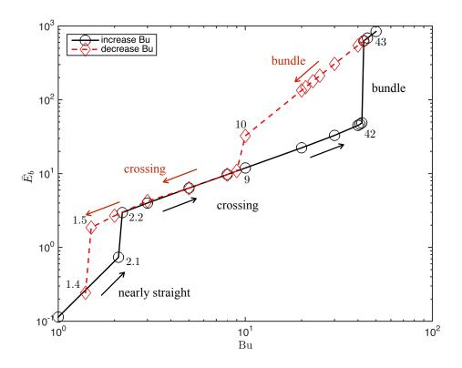
FIG. 7. Dimensionless bending energy for each filament,  $\bar{E}_b$ , as a function of the Bundling number, Bu. The black solid line displays the steady-states when increasing the values of Bu while the red dashed line shows the states obtained when decreasing Bu, showing two hysteresis loops. The critical Bu values at the transitions in the increasing branch are Bu  $\approx 2.1$  and 42, while for the decreasing branch they are Bu  $\approx 10$  and 1.5.
