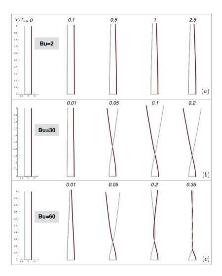
FIG. 4. Bundling of two elastic filaments as a function of time for three representative values of Bu; (a): Bu = 2, with a weakly bent final configuration; (b): Bu = 30, with a final crossing configuration; (c): Bu = 60, with a final bundled state. The bending energies corresponding to these shapes are plotted in Fig. 5. The dynamics illustrated in this figure can be visualised in the movies available in supplementary material [54].
