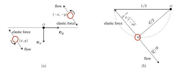
FIG. 16. (a) Setup for two-dimensional cylindrical model: two parallel rigid cylinders linked elastically to a reference position interact hydrodynamically; (b) Geometric calculation of magnitude of forces (see text for details).
