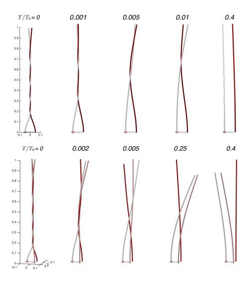
FIG. 11. Hydrodynamic unbundling of rotating filaments. Top: cases of two bundled filaments where at t = 0 the Bundling number of the filament on the left (with red dot at bottom) is switched to Bu = -50, while for the other is maintained at Bu = 50. Bottom: three filaments where the filament with the red dot at bottom is switched to Bu = -40, while for the other two are maintained at Bu = 40.
