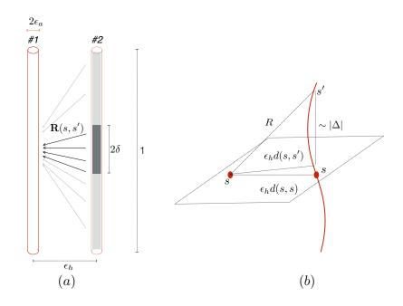
FIG. 3. (a) Illustration of the mathematical method used to compute hydrodynamic interactions. The integration domain is divided into a local region of length  $2\delta$  (dark gray) and non-local region (light gray); (b) Geometric relations between d(s, s')and R: R is the distance between two points on the two filaments;  $\epsilon_h d(s, s')$  is its projection in x - y plane;  $\epsilon_h d(s, s)$  is the local separation distance between two points at the same arclength s.
