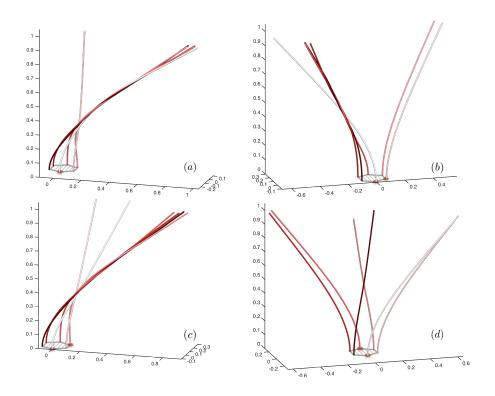
FIG. 12. Steady unbundled states for N = 6 filaments. Filaments with a red dot at their base have negative rotation and Bu = -40 while all other ones are maintained at Bu = 40. Counter-rotation is implemented for: (a) one filament; (b) two adjacent filaments; (c) two every-other filaments; (d) two opposite filaments.
