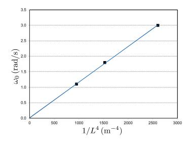
FIG. 20. Plot of critical angular velocity,  $\omega_0$ , versus  $1/L^4$  for first crossing instability. For all data, filament radius a = 0.42 mm, filament separation  $h_0 = 10$  mm, elastic modulus of filaments G = 1 GPa and viscosity of silicon oil of 12.8 Pa.s (at 20°C). Straight line is linear best fit (R = 0.9993) to the data giving a constant critical Bu = 2.14.
