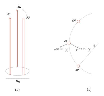
FIG. 8. (a) Configuration of N filaments symmetrically distributed along a circle of diameter  $h_0$ ; (b): Top view of the N filament configuration;  $\mathbf{v}^{(j)\to(i)}$  denotes the velocity generated by *j*th filament near the *i*th one while  $\theta = 2\pi/N$ . By exploiting the symmetries of the setup, the net flow generated by *j*th (j = 2, 3...N) and (N + 2 - j)th filaments is independent of *j*.
