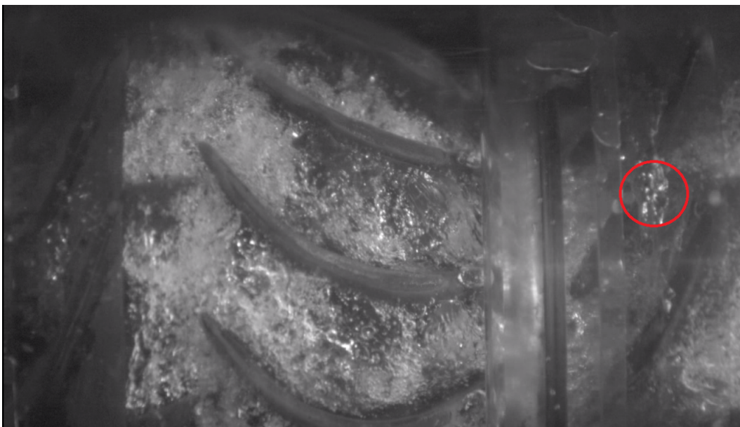
Figure F.8 Radially separated flow in the impellers and diffusers. \Phi^* = 1.54 , \lambda_0 = 9.5\% , Impellers 1-2, 7200 fps.
