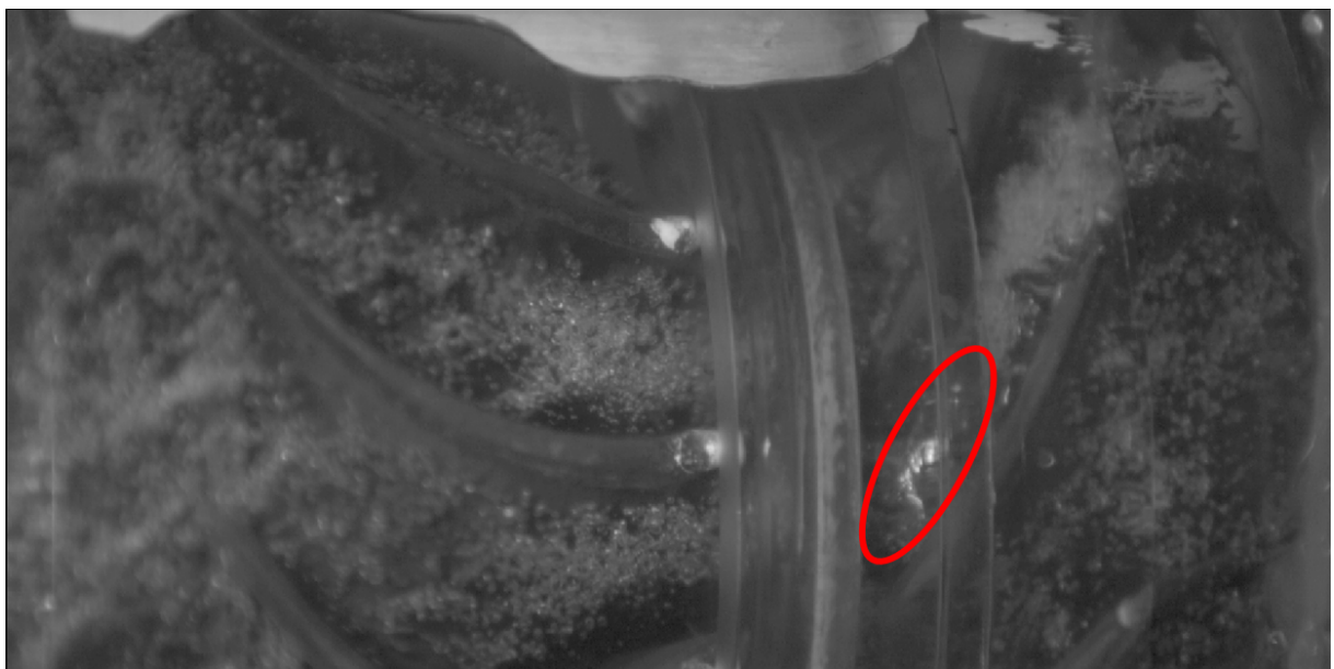
Figure F.5 Bubbly flow with intermittent gas pocket in the impeller. \Phi^* = 1 , \lambda_0 = 5\% , Impellers 3-4, 7200 fps.
