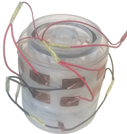
Figure 2.8 Picture of the copper electrodes and wires attached to the pump casing.
