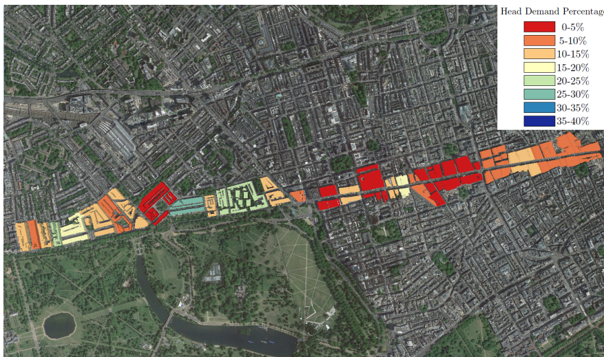
Figure 26. Map of the building cluster's annual heat demand compared to the heat extracted from the vertical boreholes in the Central Line in percentage.
