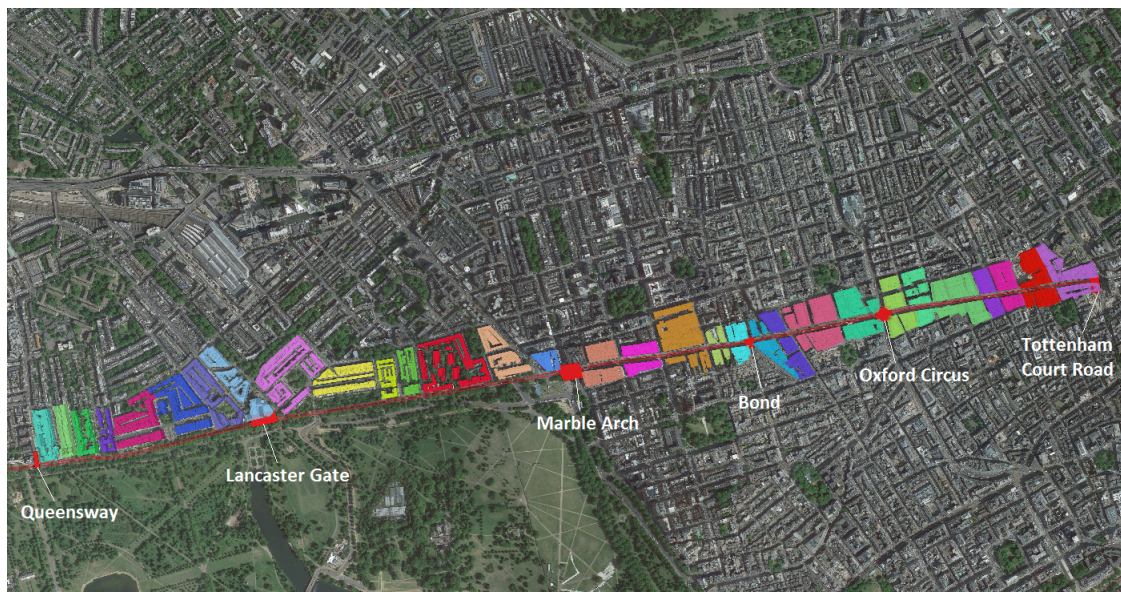
Figure 20. Map showing a section of the Central Line, and the 31 building clusters surrounding the tunnels, where each cluster is marked by a distinct color, and they are numbered from 1 to 31 from the left to the right side of the map.
