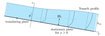
FIGURE 4. A plate inclined at an angle  $\theta$ . The effect of streamwise gravity is subdominant for x = O(1) provided that  $\theta \ll 1$ , so that the perturbation solution is valid there. Gravity eventually becomes important and the flow develops into a Nusselt film, with velocity given by (4.1) and depth  $h_{\infty}$  given by (4.2).
