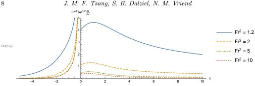
FIGURE 2. Plots of  $Fr^{-2}\partial p^{(1)}/\partial x$  against x for (a)  $Fr^{2} = 1.2$ , (b)  $Fr^{2} = 2$ , (c)  $Fr^{2} = 5$ , (d)  $Fr^2 = 10$ , from the real part of (3.12). Note that dividing by  $Fr^2$  allows a comparison with the other terms in (3.3) (see text for details).
