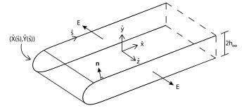
FIGURE 1. Sketch of the sheet, with the  $\hat{z}$ -axis parallel to the edge. The far-field thickness  $2h_{\infty}$ , the longitudinal strain rate E and the fluid parameters  $\mu$  and  $\gamma$  are uniform.
