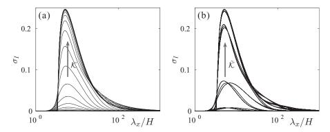
FIG. 4. Growth rate  $\sigma_I = \operatorname{Im}(\sigma)$  of the most amplified modes given by (21). (a) Isotropic case with  $\Phi_{xy} = 1$  and h/H = 1. Curves are shown for  $(\sqrt{K_x K_y}/H^2)(UH/\nu) = 10^{[-2(0.4)6]}$ . (b) Anisotropic case obtained using all possible combinations of  $h/H = 10^{[-1,0,1]}$  and  $\Phi_{xy} = 10^{[-3(1)3]}$ . Curves are shown for  $\tilde{\mathcal{K}} = 10^{[-2(1)6]}$ .
