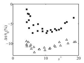
FIG. 1. Drag reduction  $DR = -\Delta \tau / \tau_0$  of the seal fur surface from Itoh *et al.* [5]:  $\Delta$ , seal fur;  $\blacksquare$ , trapezoidal flat-peak riblets, also from Itoh *et al.* [5]. For the seal fur, the wavelength identified by Itoh *et al.* by analogy with the riblet pitch  $s^+$  has been used to express their results in terms of a viscous length scale.
