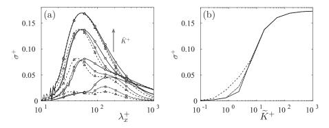
FIG. 6. (a) Growth rate  $\sigma^+ = \alpha^+ \mathrm{Im}(c^+)$  of the most amplified mode as a function of the longitudinal wavelength  $\lambda_x$ : ——,  $\Phi_x = 10^{-3}$  and  $h^+ = 10$ ; ——,  $\Phi_x = 10^3$  and  $h^+ = 10$ ;  $\Delta$ ,  $\Phi_x = 1$  and  $h^+ = 1$ ;  $\infty$ ,  $\Phi_x = 1$  and  $\Phi_x = 1$ .
