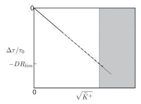
FIG. 7. Schematic summarizing the initial linear behavior of  $DR = \Delta \tau / \tau_0$  for low permeability. The hatched area represents the region  $\tilde{K} > \tilde{K}_{KH}$ , where the drag reducing effect is destroyed by the appearance of Kelvin-Helmholtz rollers.
