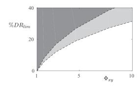
FIG. 8. Limit for the maximum drag reduction achievable as a function of the anisotropy ratio of the permeable layer  $\Phi_{xy}$ . The dashed lines denote Eq. (26) for  $\tilde{K}_{KH}^+ = 5$  and 10, and  $\xi = 1$ . The light gray shaded region indicates the range for which Kelvin-Helmholtz rollers are expected to appear. The dark gray shaded region indicates the range for which the Kelvin-Helmholtz rollers would be fully developed.
