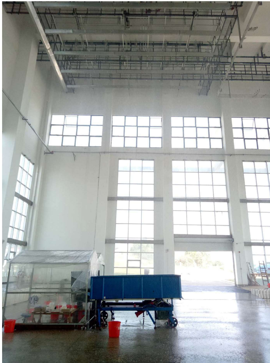
Photograph (b): the rainfall simulator, the steel flume and the plastic tent at one end of the flume was for collecting runoff water samples
