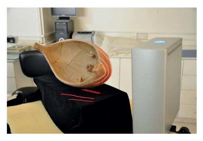
Figure 9.2. The 3D scanning of the Kazaphani model boat.
