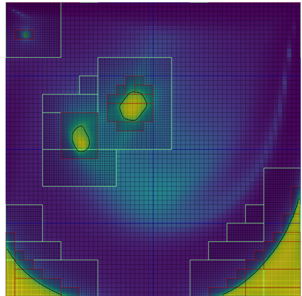
FIG. 9. Illustration of spatio-temporal adaptive mesh refinement for tracking the development of the yield surface, with Re = 1000 and Bi = 1 . The coarsest grid discretises with cell spacing 1/64 , but the two refinement layers ensure that the effective resolution near the yield surface is 1/256 . Multimedia view: https://doi.org/10.1063/1.5049202.1
