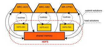
Figure 4: HDFS management for Generalized Island Model in Hadoop architecture (MRC-GIM)
