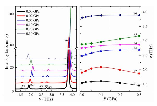
Figure 2: DFT-predicted infrared spectrum of ZIF-8 as a function of pressure  $(0.0-0.30\,\mathrm{GPa})$  in the terahertz region (left) and the evolution of the IR-active vibrational modes as a function of pressure (right).
