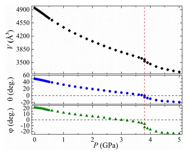
Figure 5: Volume V, imidazolate linkers "gate-opening" rotation angle  $\varphi$ , and  $\mathbf{ZnN}_4$  tetrahedra tilting angle  $\theta$  as a function of pressure.
