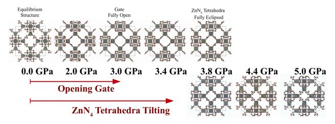
Figure 4: Pressure-induced structural changes through the first-order phase transition and up to 5 GPa in pristine ZIF-8.
