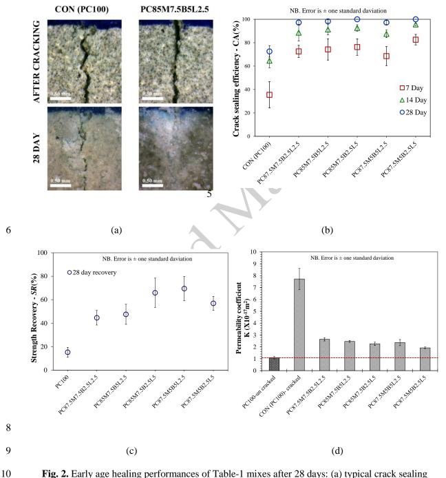
**Fig. 2.** Early age healing performances of Table-1 mixes after 28 days: (a) typical crack sealing image, (b) crack sealing efficiency, (c) strength recovery percentage, and (d) gas permeability coefficient improvement.
