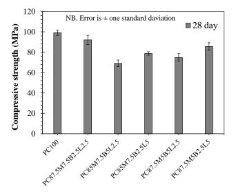
Fig. 1. The compressive strength of 28-day cubes.
