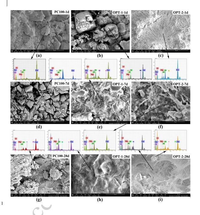
**Fig. 9.** Typical SEM images and EDX elemental composition of the self-healing materials after the 28 day healing of each cracking age samples: 1 day cracking age samples, (a) PC100, (b) OPT1 and (c) OPT-2; 7 day cracking age samples, (d) PC100, (e) OPT1 and (f) OPT-2; and 28 day cracking age samples, (g) PC100, (h) OPT1 and (i) OPT-2.
