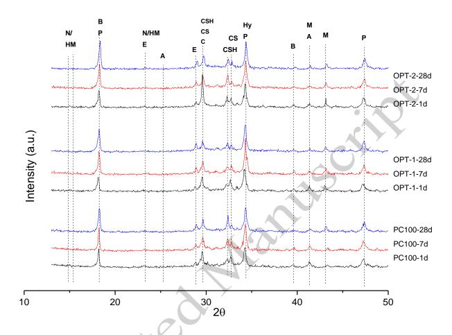
**Fig. 4.** XRD graphs of the cement mixes on different cracking ages (1 day, 7 day and 28 day) (Graph notations: A= Anhydrate, E= Ettringite, Hy= Hydrotalcite, N/HM= Nesquehonite/Hydromagnesite, B=Brucite, C= Calcite, CSH= C-S-H, CS= C<sub>2</sub>S and C<sub>3</sub>S, P= Portlandite, M= MgO/MgCO<sub>3</sub>).
