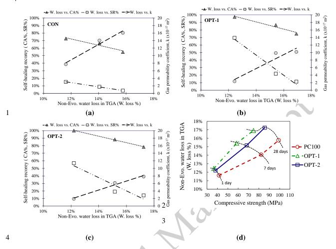
**Fig. 10.** Overall cracking age impact on the self-healing recovery and gas permeability: (a) PC100, (b) OPT-1, (c) OPT-2, and (d) Compressive strength relation to non-evaporative water loss in TGA.
