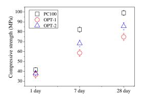
Fig. 3. Compressive strength development after 28 days
