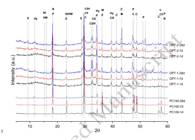
**Fig. 8.** XRD diagrams of the self-healing materials (Graph notations: E= Ettringite, Hy= Hydrotalcite, N/HM= Nesquehonite/Hydromagnesite, B=Brucite, C= Calcite, CSH= C-S-H, CS= C<sub>2</sub>S and C<sub>3</sub>S, P= Portlandite, M= MgO/MgCO<sub>3</sub>).
