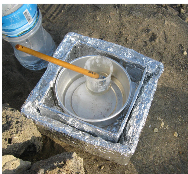
Figure 3 Home-made insulated box with layers of aluminium foil, cardboard, and cotton wadding. Photo: E. Ohara Anderson.
