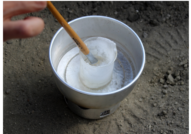
Figure 1 CDD melted in the ‘double boiler’ in the field. Photo: R. Peters.
