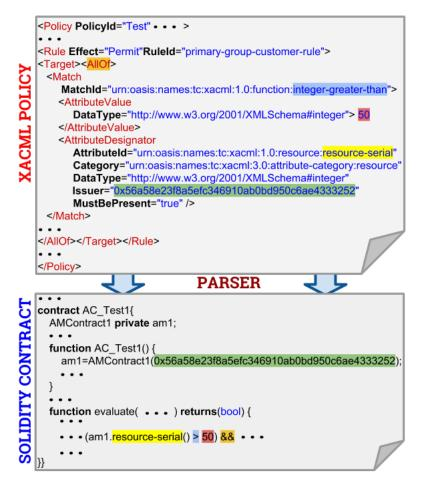
Figure 3: Simplified XACML to Solidity parser example.
