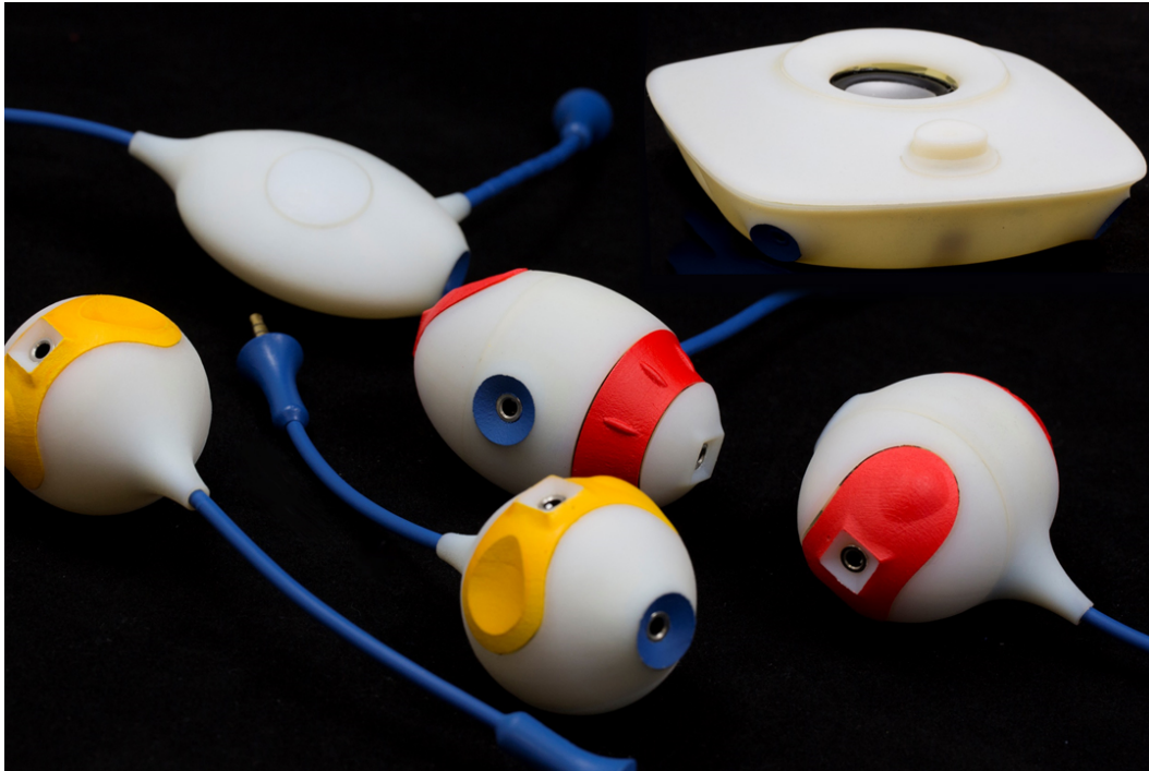
Figure 4: Torino beads (left to right): Pause (yellow), Loop (white), Play (red), Hub (square).
