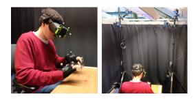
Figure 1: User shown typing in mid-air with HMD, hand and fingertip tracking markers (left). OptiTrack camera setup for precision marker tracking (right).
