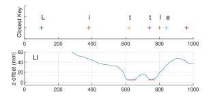
Figure 16: Illustration of a double tap executed with the left index finger while typing the word 'little'.
