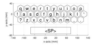
Figure 3: The keyboard layout used in the experiment. Note the reduced set of punctuation.
