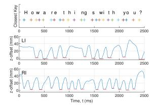
Figure 14: The z-offset resolved into the keyboard frame for the trace shown in Figure 11. The depth, frequency and duration of touches can be easily observed. LI: left index (middle), RI: right index (bottom).
