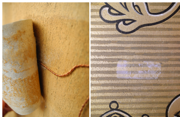
Figure 12 (left) CDD acting as a solvent and transporting colour particles at the Fischerweber farmhouse; (right) slowly subliming CDD after the installations at Neuschwanstein Castle have been dismantled. No surface changes are visible.
