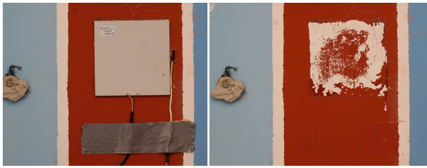
Figure 1 A conventional mounting system in a building at the Fraunhofer test facility, Holzkirchen: (a) during installation; (b) showing the losses and residues caused by removal.
