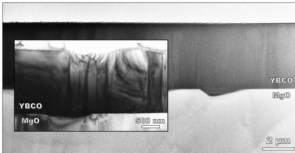
*Fig. 8.12 TEM images of a LPE grown YBCO on MgO substrate. The inset shows an enlargement of an interfacial disturbance.*
