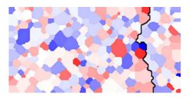
**Figure 9.** Schematic of a coated conductor with various grain alignments showing a possible limiting path perpendicular to the current flow direction.
