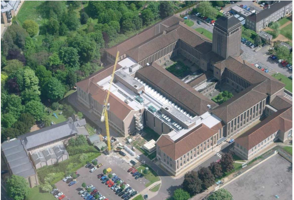
Aerial view of the Library showing the completed Phase 5 extension (immediately behind the crane) and the gap awaiting Phase 6
