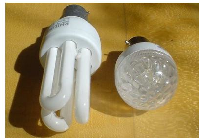
Figure 9.4. Philips 11 W alongside Omicron 1.3 W LED bulb.
