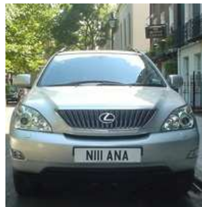
Figure 20.1. This chapter's starting point: an urban luxury tractor. The average UK car has a fuel consumption of 33 miles per gallon, which corresponds to an energy consumption of 80 kWh per 100 km. Can we do better?
