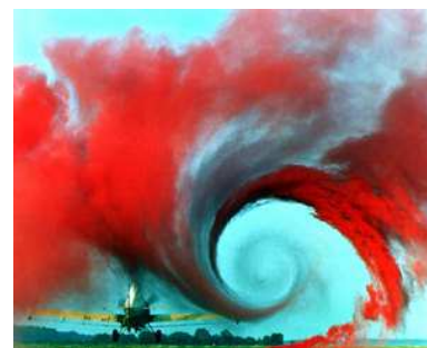
Figure C.4. Air flow behind a plane. Photo by NASA Langley Research Center.
