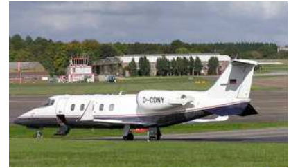
Figure C.10. “Fasten your cufflinks.” A Bombardier Learjet 60XR carrying 8 passengers at 780 km/h has a transport cost of 150 kWh per 100 passenger-km. Photograph by Adrian Pingstone.
