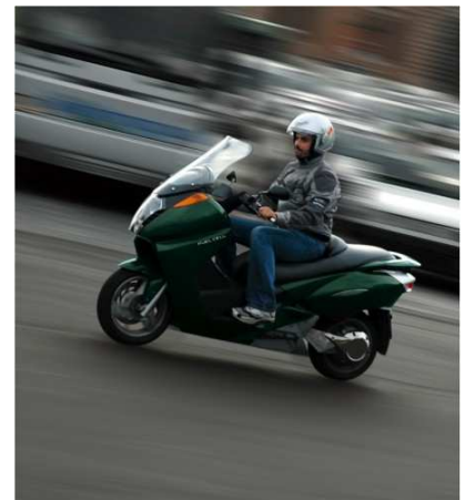
Figure 20.44. Vectrix: 2.75 kWh per 100 km . Photo from www.vectrix.com .
