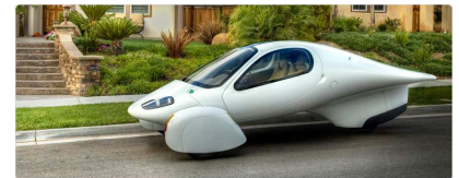
Figure 20.40. The Aptera. 6 kWh per 100 km . Photo from www.aptera.com.
