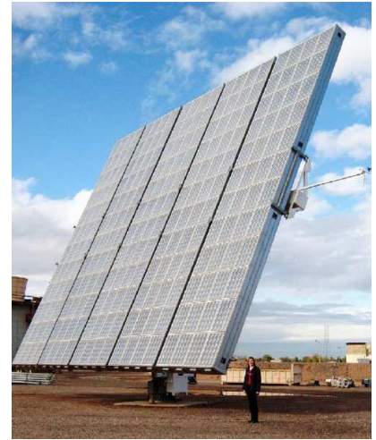
Figure 25.9. A 25 kW (peak) concentrator photovoltaic collector produced by Californian company Amonix. Its 225 \text{ m}^2 aperture contains 5760 Fresnel lenses with optical concentration \times 260 , each of which illuminates a 25%-efficient silicon cell. One such collector, in an appropriate desert location, generates 138 kWh per day – enough to cover the energy consumption of half an American. Note the human providing a scale. Photo by David Faiman.
