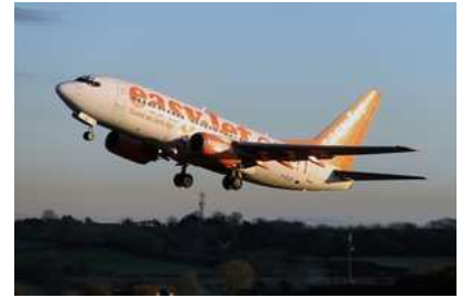
Figure C.11. Boeing 737-700: 30 kWh per 100 passenger-km. Photograph © Tom Collins.
