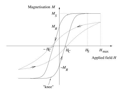
Figure 4.1: A major hysteresis loop (solid line), showing the coercive field  $H_C$ , remanence  $M_R$  and saturation magnetisation  $M_S$ , and a minor loop (dashed line). The arrows show the direction of magnetisation.
