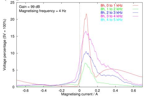
Figure 8.26: 600°C, 8 hour tempering: signals obtained from different frequency ranges.
