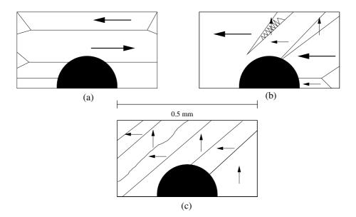
Figure 3.8: Domain structures in Fe-3.5 wt. % Si, observed by Bitter technique (Seeger *et al.*, 1969). (a) zero field; (b), (c) field increasing. The large black area is a dark area appearing on the original micrographs, perhaps due to surface damage.
