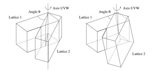
Figure 7.1: The angle-axis pair  $\theta < UVW >$  characterises the crystallographic orientation between the two grains but the actual boundary can be anywhere. After Randle and Engler, 2000.
