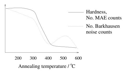
Figure 4.6: Effect of annealing temperature on mechanical and magnetic properties of deformed nickel (Ranjan *et al.*, 1987c).
