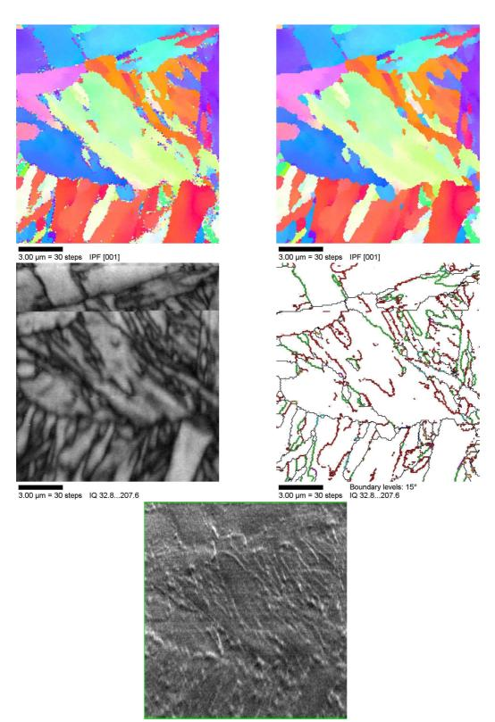
Figure 7.24: 2<sup>1</sup>/<sub>4</sub>Cr1Mo steel, 600 °C, 256 hours tempering - 189 -
