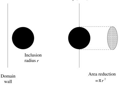
Figure 3.2: Energy reduction by intersection of inclusion with domain wall (Kersten, 1943).
