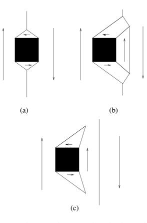
Figure 3.4: Interactions between domain wall and cubic inclusion with spikes (after Craik and Tebble, 1965): (a) domain wall at local energy minimum, (b) movement of main domain wall, (c) detachment of wall from inclusion.
