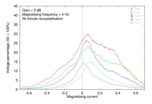
Figure 10.23: BN signals from samples heated at 1380°C for 30 minutes, measured in longitudinal direction. Line 4 was measured on the recrystallised/unrecrystallised boundary, line 5 in the unrecrystallised region, and the others in the recrystallised region.
