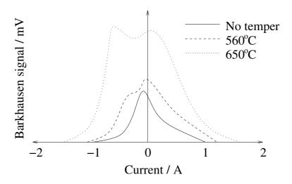
Figure 4.14: Changes in BN peak size and shape due to tempering (Buttle *et al.*, 1987c).
