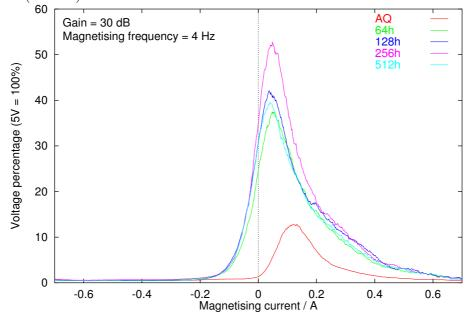
Figure 8.10: BN voltage versus magnetising current for samples tempered at  $600^{\circ}$ C (64–512 h).
