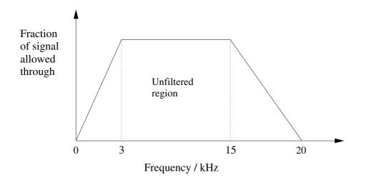
Figure 8.21: Frequency filter in 'rollscan' mode (Blaow, personal communication).
