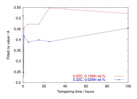
Figure 5.13: Relationship of Model 2 fitting parameter  $\Delta x$  with tempering time for two steels of similar composition.
