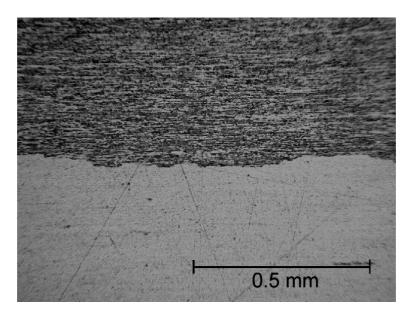
Figure 10.5: Optical micrograph showing recrystallised and unrecrystallised regions.
