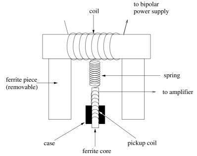
Figure 8.3: Schematic diagram of BN sensor.
