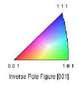
Figure 7.5: Colour-coded pole figure key for orientation maps. Colour corresponds to orientation of [100] specimen axis with respect to crystal axes [001], [111] and [101].
