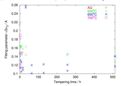
Figure 9.8:  $\langle S \rangle_2$  versus tempering time for Model 2,  $2\frac{1}{4}$ Cr1Mo steel.
