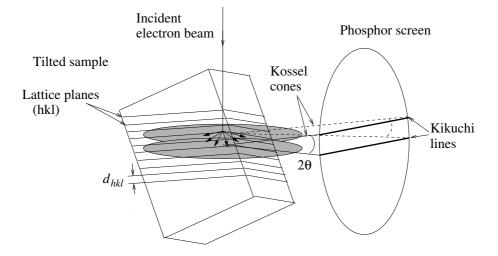
Figure 7.2: Geometry of electron backscatter diffraction; after Randle and Engler, 2000.
