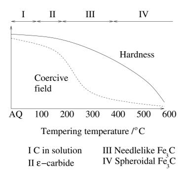
Figure 4.13: Changes in hardness and coercive field associated with different tempering times (Kameda and Ranjan, 1987a).
