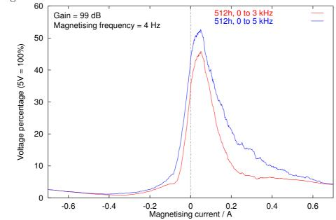
Figure 8.28: 600°C, 512 hour tempering: comparison of 0–3 kHz and 0–5 kHz ranges.
