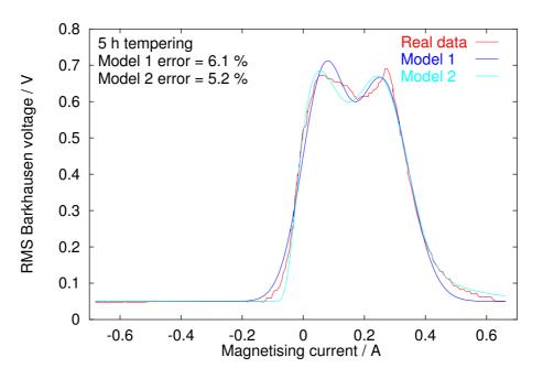
Figure 5.5: Fitting of data for plain-carbon steel tempered for 5 h.
