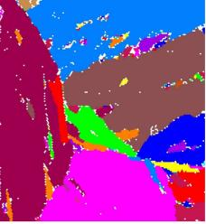
3.00 µm = 30 steps Unique Grain Color 600°C, 256 hour tempered; Figure 7.23
