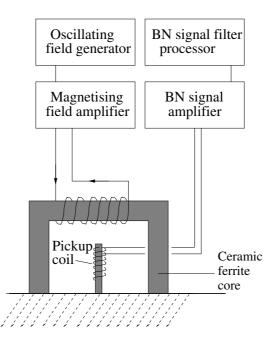
Figure 8.2: Schematic diagram of BN measurement equipment (after Blaow, 2001).
