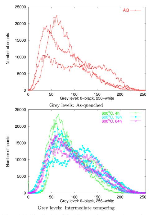
Figure 7.32: Grey levels in AQ and intermediate tempering samples.
