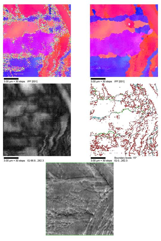
Figure 7.21: 2<sup>1</sup>/<sub>4</sub>Cr1Mo steel, 600 °C, 128 hours tempering - 186 -
