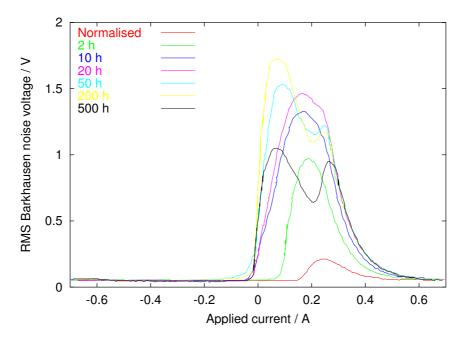
Figure 5.15: Real BN data from tempered  $2\frac{1}{4}$ Cr1Mo power plant steel. Data from Moorthy *et al.*, 1998.
