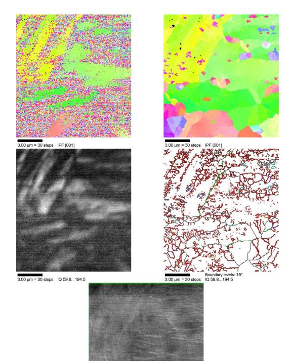
Figure 7.8:  $2\frac{1}{4}$ Cr1Mo steel, as-quenched - 173 -
