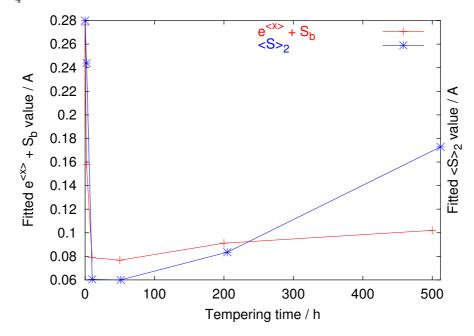
Figure 5.18: Model 2 fitting parameters  $e^{\langle x \rangle} + S_b$  and  $\langle S \rangle_2$  versus time for 9Cr1Mo steel.
