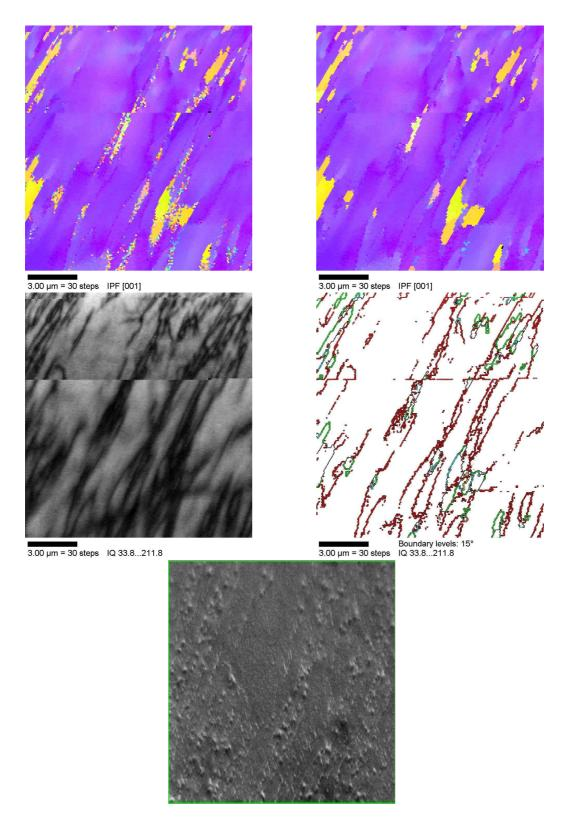
Figure 7.22: 2<sup>1</sup>/<sub>4</sub>Cr1Mo steel, 600 °C, 256 hours tempering - 187 -
