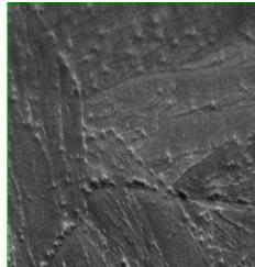
Figure 7.23: 2<sup>1</sup>/<sub>4</sub>Cr1Mo steel, 600 °C, 256 hours tempering - 188 -
