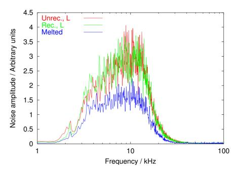
Figure 10.15: Frequency spectra from unrecrystallised, recrystallised and melted PM2000 magnetised at 4 Hz.
