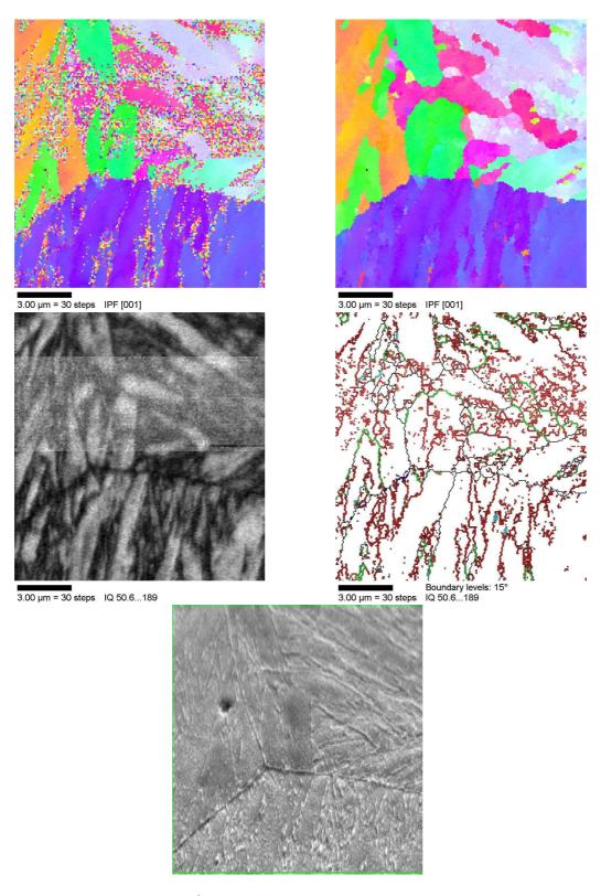
Figure 7.15: 2<sup>1</sup>/<sub>4</sub>Cr1Mo steel, 600 °C, 16 hours tempering - 180 -
