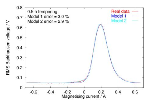
Figure 5.3: Fitting of data for plain-carbon steel tempered for 0.5 h.
