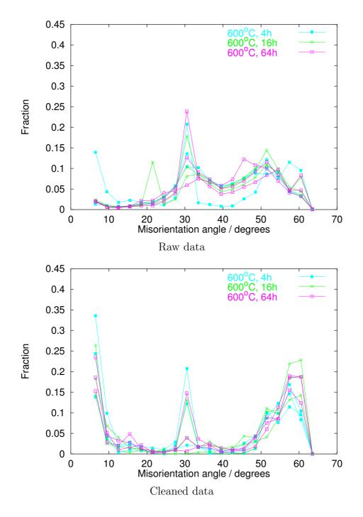
Figure 7.27: Misorientation angle distributions for intermediate tempering times (4–64 hours).
