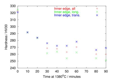
Figure 10.9: Hardness in longitudinal and transverse directions for inner edge.
