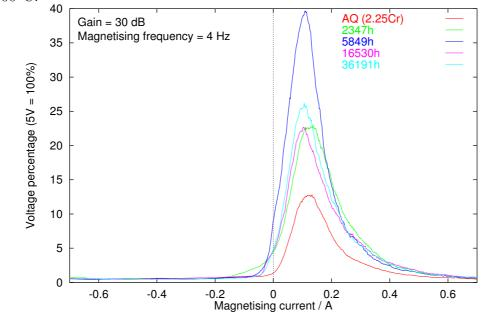
Figure 8.12: BN voltage versus magnetising current for 11Cr1Mo wt. % specimens.
