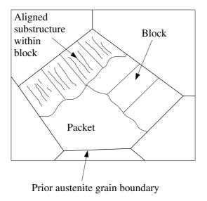
Figure 2.4: Levels of structure in martensite, (Marder and Marder, 1969).
