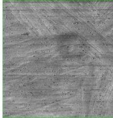
Figure 7.7:  $2\frac{1}{4}$ Cr1Mo steel, as-quenched
