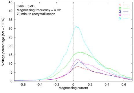
Figure 10.24: BN signals from samples heated at 1380°C for 70 minutes, measured in longitudinal direction. Lines 2 and 4 are signals measured along grain boundaries, and the others come from within the grains.
