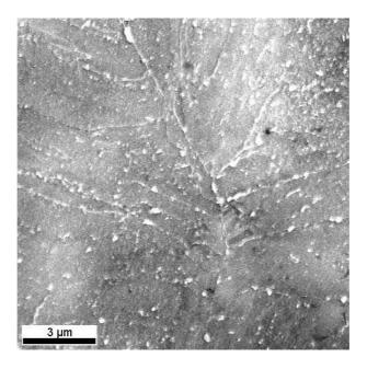
Figure 6.26: SEM micrograph of  $2\frac{1}{4}$ Cr1Mo steel tempered at 700°C for 1 hour.
