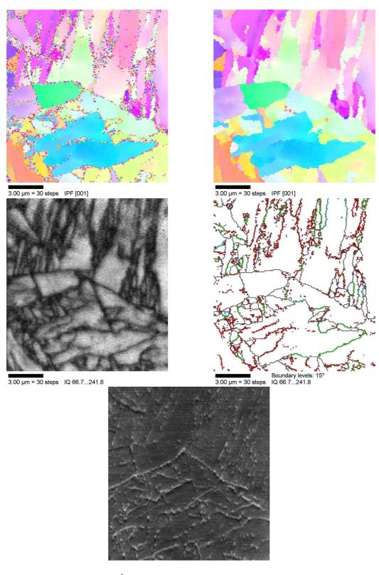
Figure 7.19: 2<sup>1</sup>/<sub>4</sub>Cr1Mo steel, 600 °C, 128 hours tempering - 184 -
