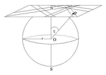
Figure 7.3: The Kikuchi diffraction pattern as a gnomonic projection of angles within the crystal; after Randle and Engler, 2000.
