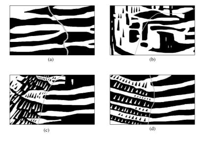
Figure 3.10: Domain structures observed at grain boundaries in Fe-3 wt. % Si by Kerr microscopy (schematic): (a), (b) low-angle boundary, (c), (d) random boundary (Kawahara *et al.*, 2000).
