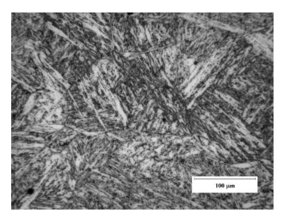
Figure 6.16: 11 wt. % Cr steel heated for 2347 hours at 550°C during creep test.
