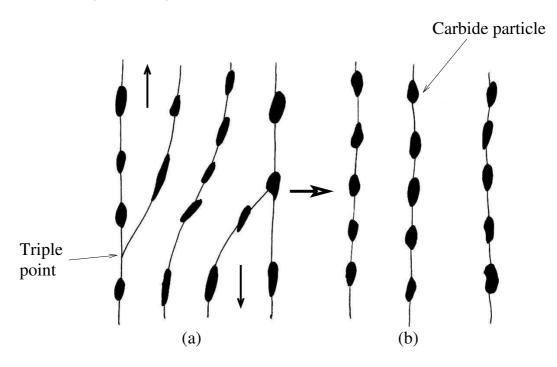
Figure 2.8: Lath coalescence: Triple points migrate and lath boundaries coalesce (a) to give a coarser structure (b). After Abe, 1999.
