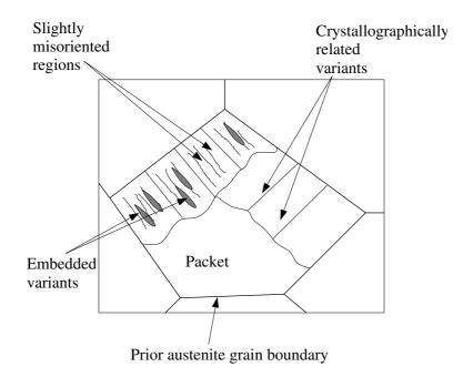
Figure 7.34: Possible levels of structure in 2.25Cr1Mo wt. % martensite, as deduced from OIM observation.
