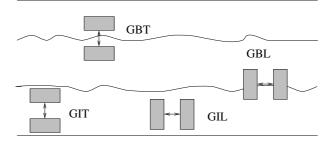
Figure 10.17: Positions in which Barkhausen signal was measured. GB, GI are grain boundary and grain interior; L and T are longitudinal and transverse.
