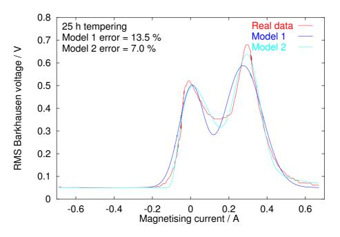
Figure 5.7: Fitting of data for plain-carbon steel tempered for 25 h.
