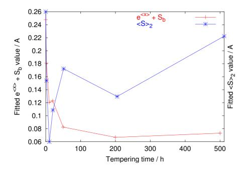
Figure 5.17: Model 2 fitting parameters  $e^{\langle x \rangle} + S_b$  and  $\langle S \rangle_2$  versus time for  $2\frac{1}{4}$ Cr1Mo steel.
