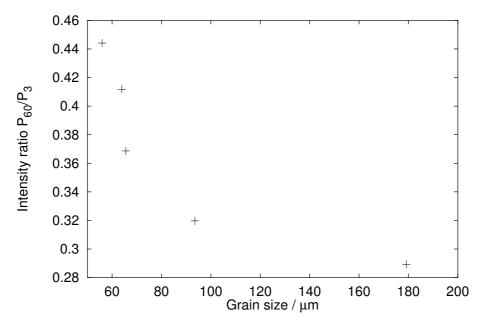
Figure 4.5: Relationship between frequency components of BN and grain size (Yamaura *et al.*, 2001).
