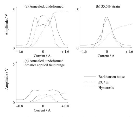
Figure 4.8: Effect of straining and changing the applied current range (and hence  $H_{\text{max}}$ ) on BN, hysteresis and dB/dt curves (Kim *et al.*, 1992).
