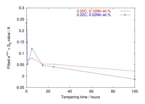
Figure 5.11: Relationship of Model 2 fitting parameters  $e^{\langle x \rangle} + S_b$  with tempering time for two steels of similar composition.
