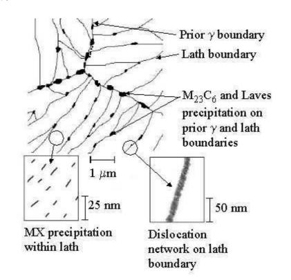
Figure 2.7 shows a typical tempered martensitic microstructure in 9–12 wt. % steel.
