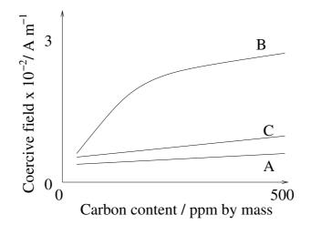
Figure 4.11: The effects of different precipitation states on the coercive field (A) carbon mostly in interstitial solution, (B) intragranular precipitates of around 0.5  $\mu$ m diameter, (C) large carbides of around 10  $\mu$ m diameter at grain boundaries (Lopez *et al.*, 1985).
