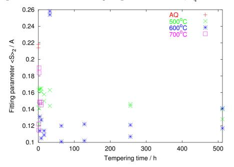
Figure 9.10:  $\langle S \rangle_2$  versus tempering time for Model 1,  $2\frac{1}{4}$ Cr1Mo steel.
