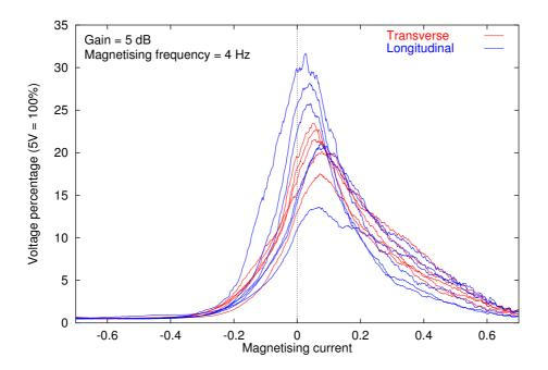
Figure 10.22: BN signals from samples heated at 1380°C for 20 minutes.
