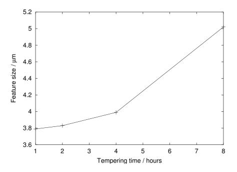
Figure 6.27: Changes in average feature spacing with tempering time at 700°C.
