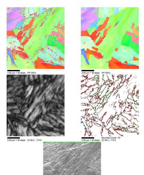
Figure 7.18: 2<sup>1</sup>/<sub>4</sub>Cr1Mo steel, 600 °C, 64 hours tempering - 183 -
