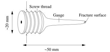
Figure 6.1: Failed creep test specimen. The arrows show the position at which the Barkhausen test specimen was cut.
