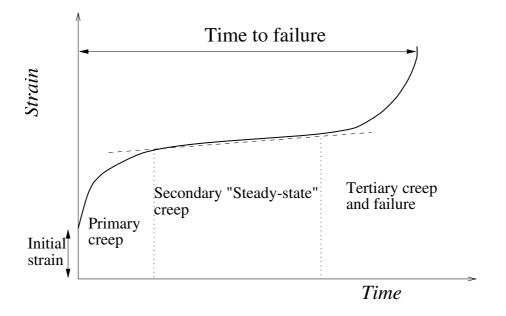
Figure 2.2: A typical strain-time curve showing the different regimes of creep (after Evans and Wilshire, 1993).
