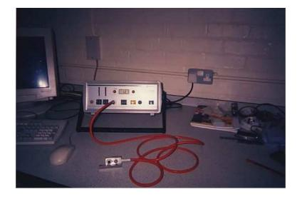
connected to a standard PC with purpose-written software installed. This is used to control the magnetising current and analyse the output.
