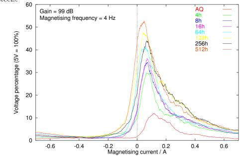
Figure 8.24: 0–5 kHz component of Barkhausen signal for  $600^\circ\mathrm{C}$  tempered steels.
