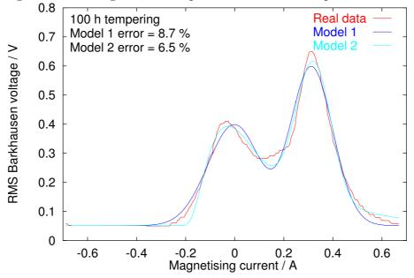
Figure 5.8: Fitting of data for plain-carbon steel tempered for 100 h.
