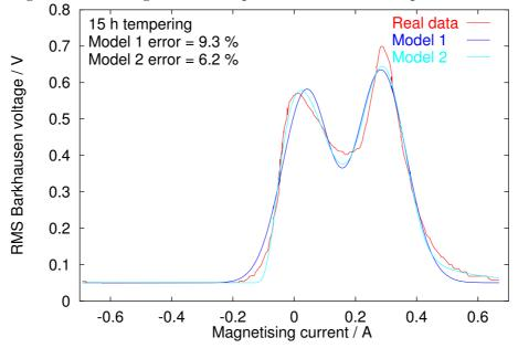
Figure 5.6: Fitting of data for plain-carbon steel tempered for 15 h.
