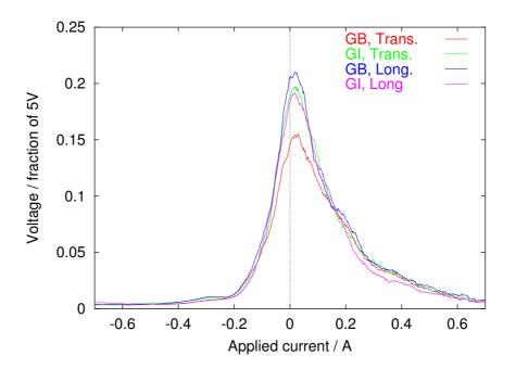
Figure 10.18: Effect on Barkhausen signal of magnetising across a grain boundary (GB) or grain interior (GI) in recrystallised PM2000.
