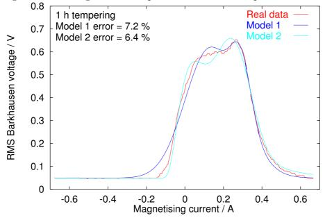
Figure 5.4: Fitting of data for plain-carbon steel tempered for 1 h.
