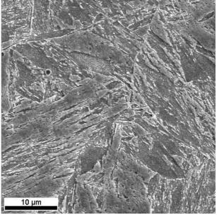
Figure 6.23: SEM micrograph of  $2\frac{1}{4}$ Cr1Mo steel tempered at 500°C for 256 hours.
