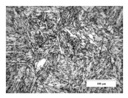
Figure 6.18: 11 wt. % Cr steel heated for 16530 hours at 550°C during creep test.
