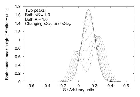
Figure 5.1: Transition between single- and double-peak behaviour
