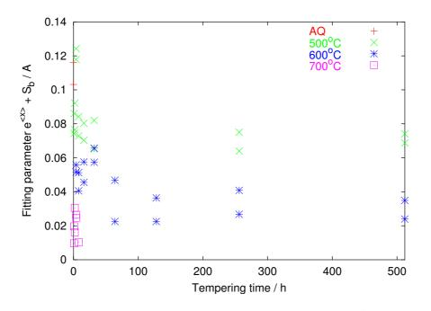
Figure 9.7:  $e^{\langle x \rangle} + S_b$  versus tempering time for Model 2,  $2\frac{1}{4}$ Cr1Mo steel.
