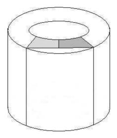
Figure 10.3: Origin of the tube-section samples, marked in grey.
