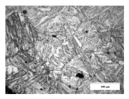
Figure 6.8:  $2\frac{1}{4}$ Cr1Mo steel tempered for 4 hours at 600°C.
