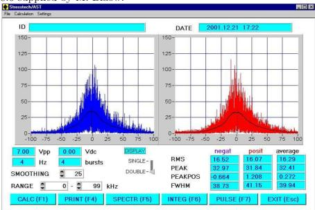
Figure 8.5: Screenshot showing the forward and reverse rectified BN.
