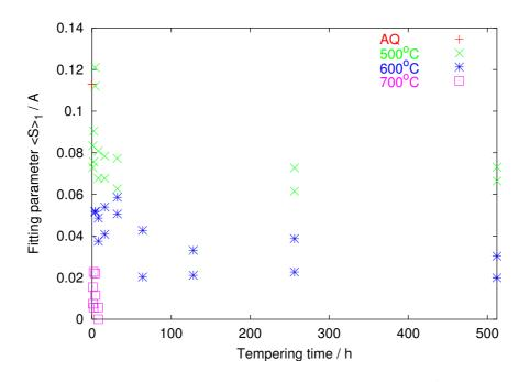
Figure 9.9:  $\langle S \rangle_1$  versus tempering time for Model 1,  $2\frac{1}{4}$ Cr1Mo steel.
