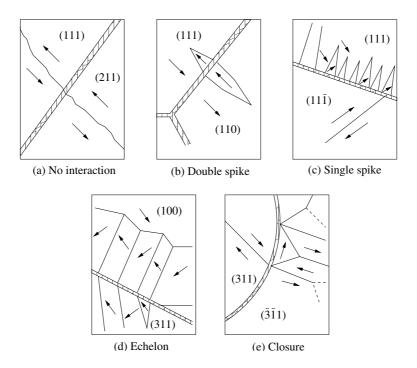
Figure 3.9: The five types of interaction between grain boundaries and domain walls, shown in order of increasing magnetic pole density at the grain boundary (Tobin and Paul, 1969).
