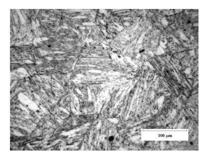
Figure 6.4:  $2\frac{1}{4}$ Cr1Mo steel tempered for 1 hour at 500°C.
