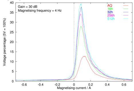
Figure 8.8: BN voltage versus magnetising current for samples tempered at  $500^{\circ}$ C (16–512 h).
