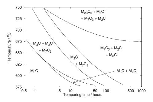
Figure 2.6: An updated version (1984) of the original Baker-Nutting carbide stability diagram (1959) for  $2\frac{1}{4}$ Cr1Mo steel, using new microanalytical techniques to identify phases (Nutting, 1999).
