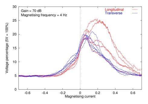
Figure 10.19: BN signal from unrecrystallised sample.
