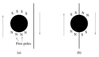
Figure 3.3: Distribution of free north (N) and south (S) poles around an inclusion (a) in the bulk (b) bisected by a domain wall (Néel, 1944).
