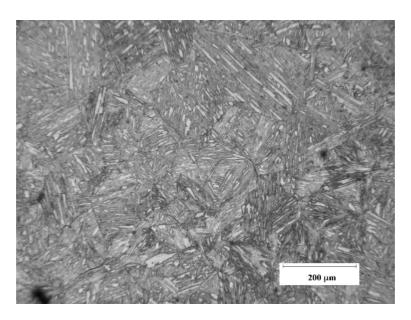
Figure 6.2: As-quenched microstructure of  $2\frac{1}{4}$ Cr1Mo steel.
