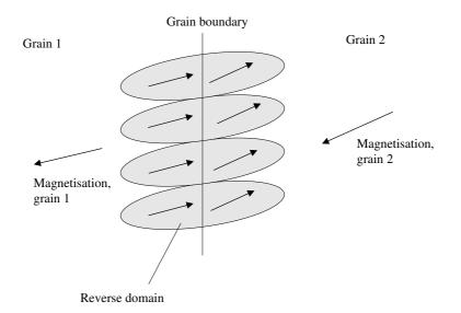
Figure 3.6: Reverse domain creation at a grain boundary (based on Goodenough, 1954).
