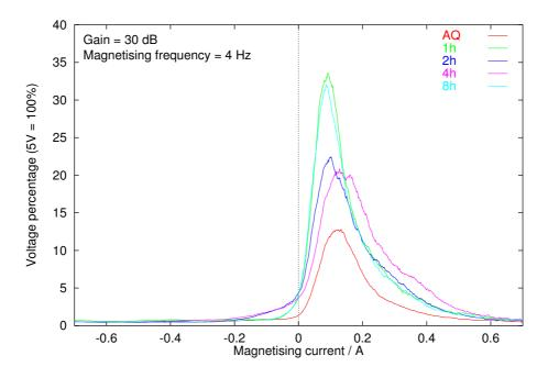
Figure 8.7: BN voltage versus magnetising current for samples tempered at  $500^{\circ}$ C (1–8 h).
