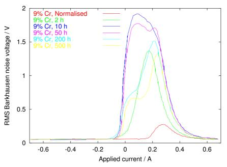
Figure 5.16: Real BN data from tempered 9Cr1Mo power plant steel. Data from Moorthy  $et \ al.$ , 1998.
