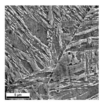
Figure 6.22: SEM micrograph of  $2\frac{1}{4}$ Cr1Mo steel tempered at 500°C for 1 hour.
