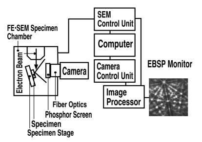
Figure 7.4: Experimental setup for SEM-based EBSD at Tohoku University. Diagram by K. Kawahara; used with permission.
