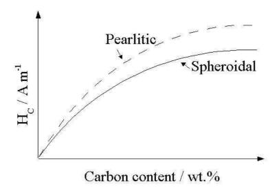
Figure 4.10: The effect of carbon content on coercive field in plain-carbon steel, for spheroidal and pearlitic microstructures (Jiles, 1988a).
