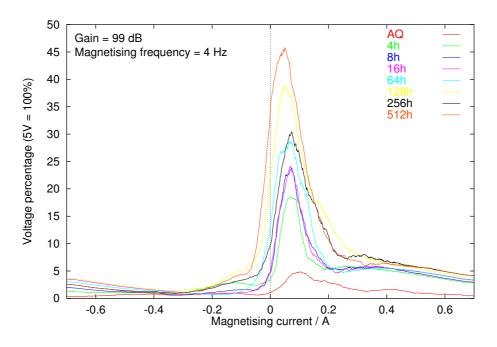
Figure 8.23: 0–3 kHz component of Barkhausen signal for  $600^{\circ}$ C tempered steels.
