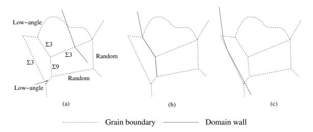
Figure 3.11: Interaction between a domain wall and grain boundaries of different types (schematic): (a) Domain wall interacts weakly with  $\Sigma$ 3 boundary because of almost perpendicular approach. Weak interaction between wall and low-angle boundary despite small impingement angle. (b) Domain wall jumps to lie parallel to  $\Sigma$ 3 boundary. (c) A jump to another  $\Sigma$  3 boundary, but the wall appears to lie beside the boundary rather than on it (Kawahara *et al.*, 2002).
