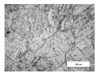
Figure 6.14:  $2\frac{1}{4}$ Cr1Mo steel tempered for 4 hours at 700°C.
