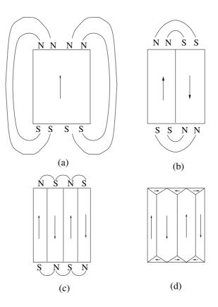
Figure 3.1: Subdivision into domains (cubic material with positive anisotropy). (a) a saturated sample, with high demagnetising energy  $E_d$ ; (b) splitting into two reduces  $E_d$ ; (c) more splitting reduces  $E_d$  further; (d) free poles eliminated by closure domains. After Kittel and Galt, 1956.
