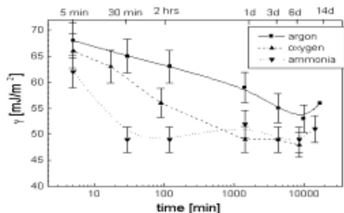
FIGURE 2. Ageing of surface free energy of PC after treatment in Ar, NH<sub>3</sub> and O<sub>2</sub> plasmas. The treatment conditions were P =100 W, U<sub>bias</sub> = -25 V, Q = 52 sccm, p = 36.5 Pa. and treatment time t = 10 min. The bars in the graph correspond to standard deviation.
