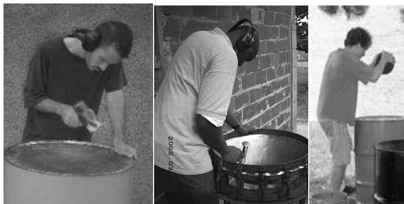
Figure 2.1: Traditional sinking of steelpan dish; Left: dishing a tight-head drum with a sledgehammer [21]; Middle: dishing a blank which is held in a jig; Right: dishing with a heavy steel ball [22]
