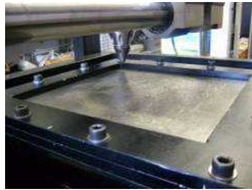
(b) Lubricated sheet-blank clamped in ISF machine
