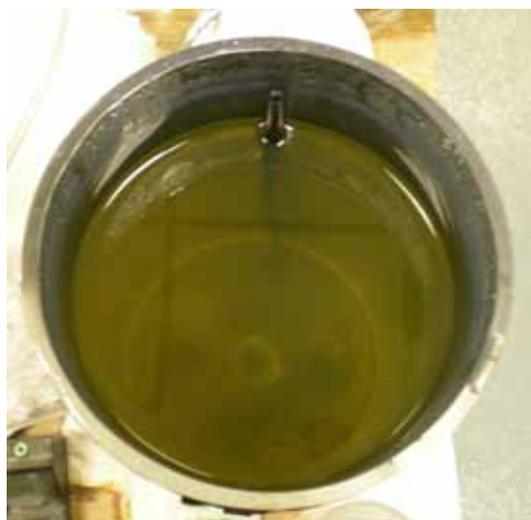
**Figure 4.9** Slightly cloudy MB solution after the first Honeycomb I experiment, indicating the precipitation of iron (III) oxides
