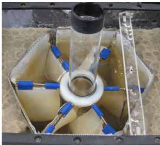
**Figure 6.18** The catalyst surface was slightly brown like the sand colour 10 months after the reactor was installed and including six sand tank experiments
