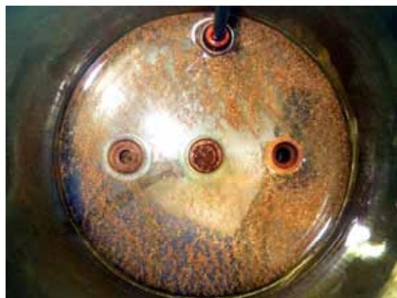
**Figure 5.7b** Plan view of the bottom of the reactor showing yellowish brown particles in the reactor, indicating precipitation of iron during the photocatalytic reaction
