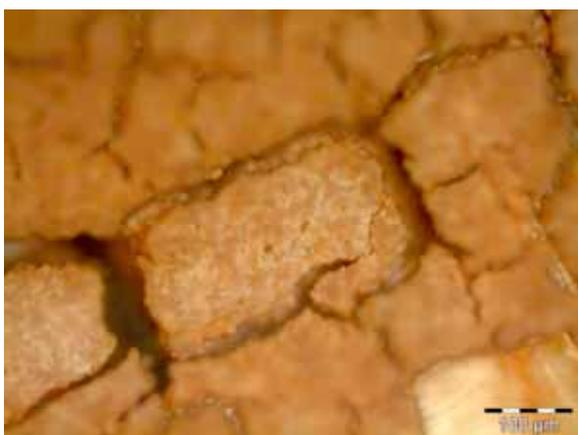
**Figure 5.18a** Microscopic image showing that the catalyst surface was yellowish brown after HIHO experiments
