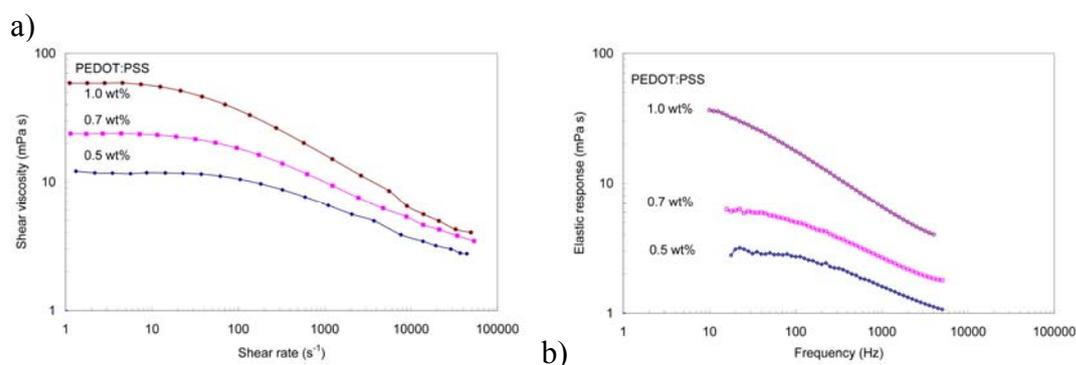
**Figure 1:** Measured values of (a) shear viscosity (mPa s) vs. shear rate (s<sup>-1</sup>) and (b) elastic response (mPa s) vs. frequency (Hz) for the PEDOT:PSS solutions indicated.
