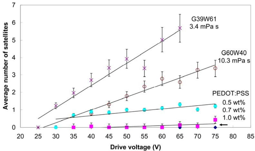
**Figure 3.** The average numbers of satellites, within 0.8 mm of the nozzle, from jetting of the PEDOT:PSS and Newtonian fluids with surfactants at a range of drive voltages. The lines are drawn to guide the eye. 1.0 wt% PEDOT:PSS had no visible satellites.
