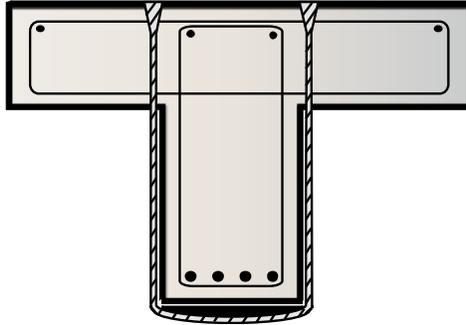
**Figure 9.** Shear strengthened T-beam (after Meier *et al*, 1997)
