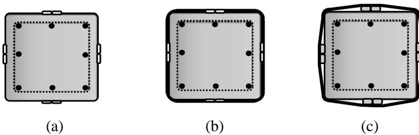
**Figure 12.** Schematic sequence for installation of continuous strap column strengthening system (a) base column with hoses on surface (b) section wrapped with CFRP straps and (c) prestressing of strap by injecting mortar into hoses
