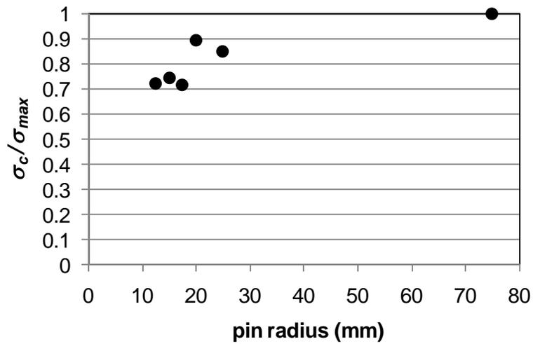
**Figure 4.** Comparison of strength of single layer strap relative to pin radius (Winistörfer 1999)
