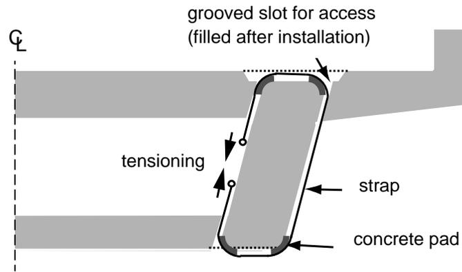
**Figure 11.** Strengthened box girder section *after* (Czaderski *et al* 2008)
