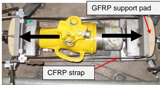
**Figure 6.** Testing of strap and GFRP pad support system
