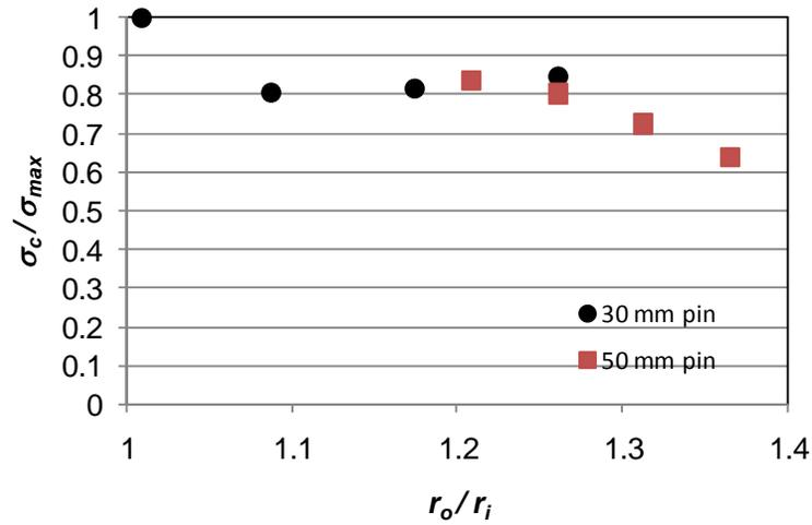
**Figure 3.** Non-laminated pin-loaded strap experimental results (Winistörfer *et al* 2001)
