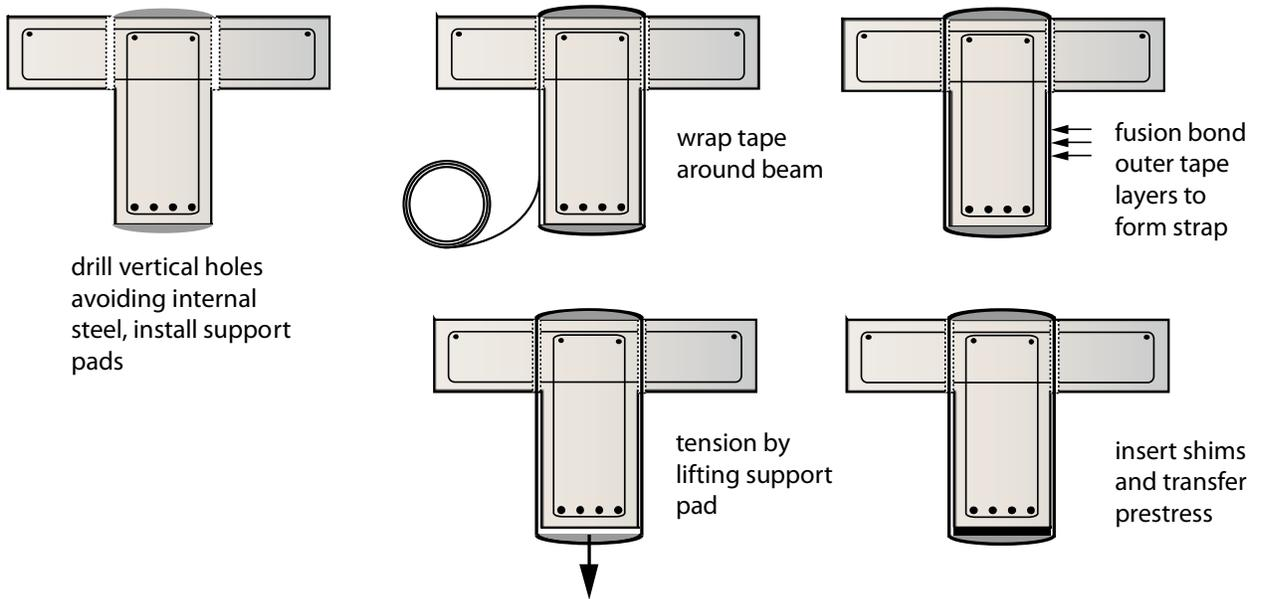
**Figure 10.** Schematic diagram of reinforced concrete web prestressing
