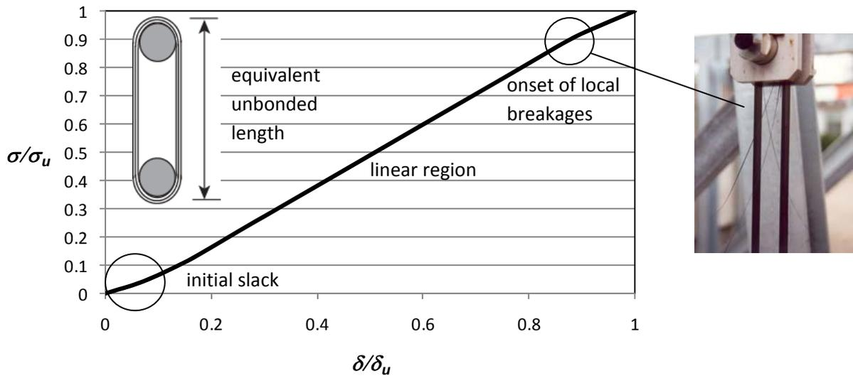
**Figure 7.** – Schematic strap load-displacement behaviour
