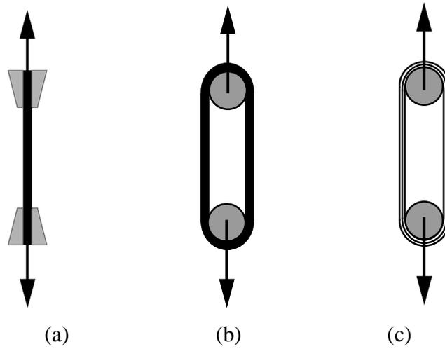
**Figure 1.** Schematic diagram of (a) straight rod or laminate (b) pin-loaded laminated loop and (c) fusion-bonded pin-loaded non-laminated loop
