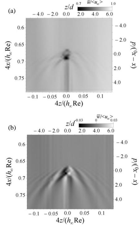
Figure 4. Spatial distribution of the surface velocity of a film flowing over a fully submerged obstacle (located at  $(x, z) = (x_0, 0)$  on the right-hand-side and top axis) at an angle of  $44^\circ$ , a flow rate of  $50 \text{ cm}^3 \text{ s}^{-1}$  (Exp. 5 in Table 1). (a) Non-dimensional time-averaged streamwise velocity; (b) non-dimensional time-averaged lateral velocity (with negative values, in darker grey, pointing to the left).
