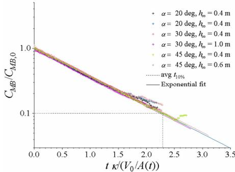
Figure 5. Normalised concentration of methylene blue dye ( $C_{MB}$ ) in the drop versus non-dimensional time. We plot the ensemble averaged data for each experiment with pluses of different colours and the corresponding exponential fits with solid lines.
