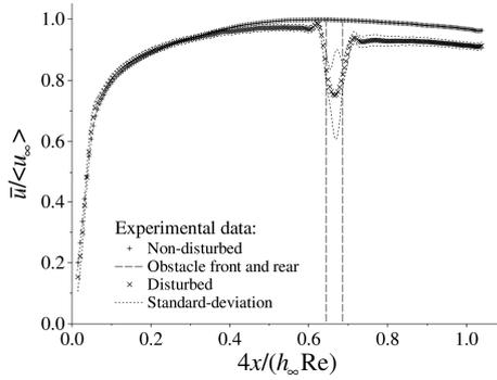
Figure 3. Non-dimensional distribution of the time-averaged surface velocity of the film (crosses) and its standard deviation (dotted curves) along the streamwise ( $x$ ) direction at a lateral ( $z$ ) location where the flow is disturbed by an obstacle (located between the two dashed vertical lines). The non-disturbed data are plotted with pluses for comparison.
