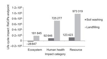
**Figure 1.** Life cycle impact estimated by ReCiPe endpoint hierarchist method. Soil washing considers impacts from excavation and soil washing/disposal and landfilling considers impacts from excavation and soil disposal
