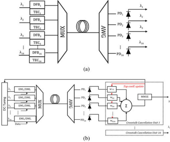
Fig. 8. 16 channel (a) Traditional. (b) MIMO DWDM.
