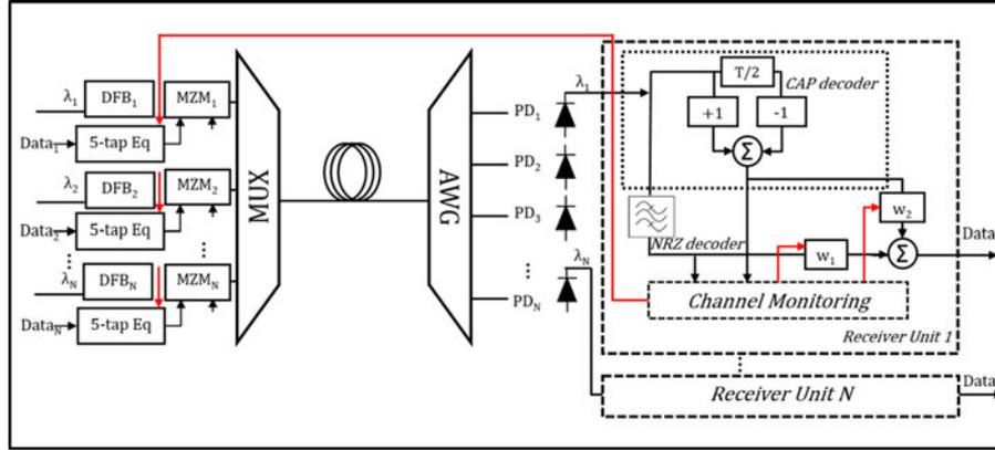
Fig. 1. 16-channel Orthogonal DWDM System Schematic.
