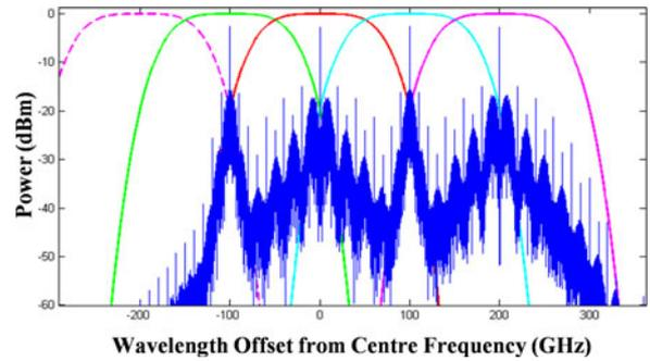
Fig. 2. Proposed AWG Profile with alternating NRZ and CAP-2Q channels.
