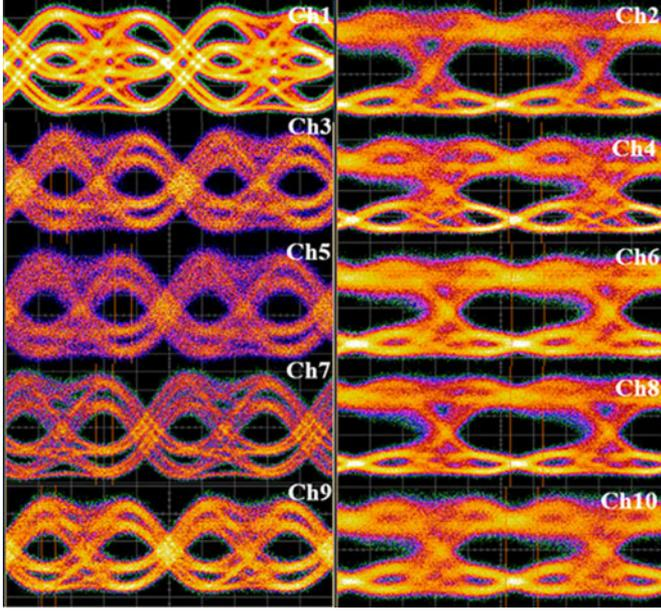
Fig. 11. Optical eye diagrams for (RHS) NRZ channels and (LHS) CAP-2Q channels (20 ps/div).
