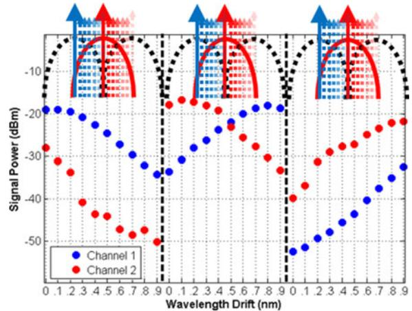
Fig. 20. Pilot tone powers versus wavelength drift for different AWG filters.
