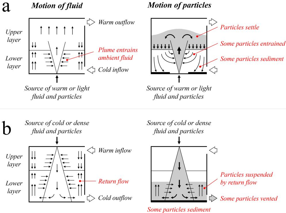
FIGURE 1. Schematics illustrating the motion of fluid and relatively heavy small particles through an upward and a downward displacement-ventilated space (a and b respectively.)
