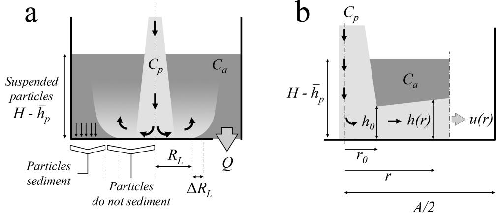
FIGURE 8. Particle-laden fountain impinging on the floor (section 3).
