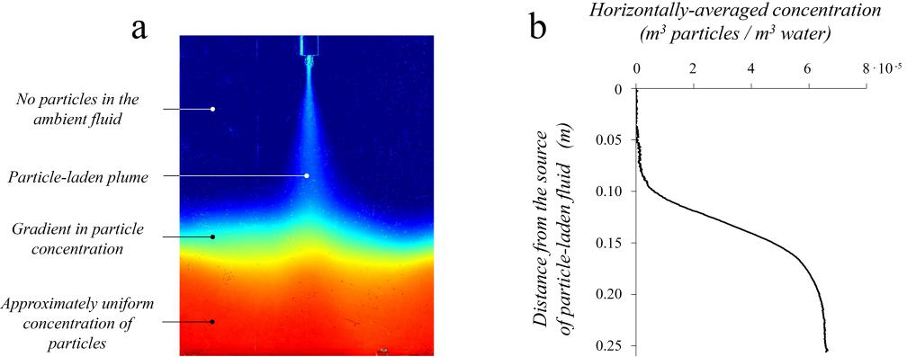
FIGURE 4. Steady-state distribution of particles in the tank in a typical experiment (experiment e, cf. table 1). Image a) illustrates the steady-state concentration of particles in the tank using false colours; image b) shows the horizontally-averaged particle concentration profile.
