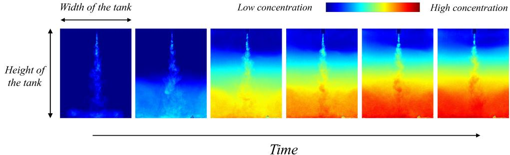
FIGURE 3. Transient concentration of particles in suspension in the tank during experiment b (cf. table 1). A series of images illustrate the concentration distribution in the tank at the following times after the beginning of the experiment: 30 seconds and 5, 28, 43, 70 and 86 minutes.
