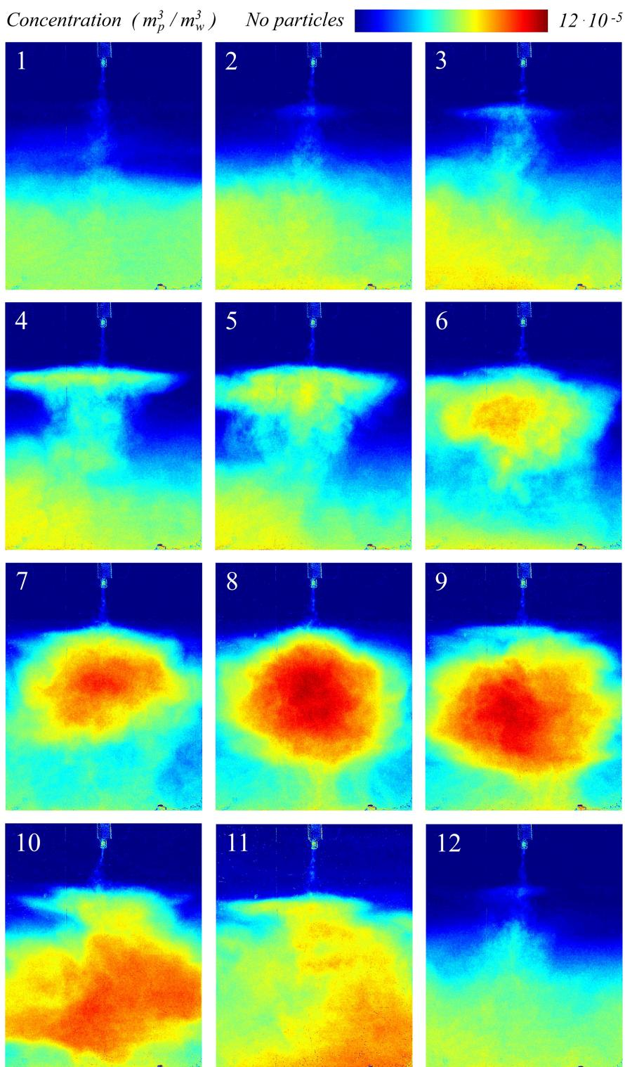
FIGURE 18. Large-scale instability observed during experiment h. Image 1 was captured 670 seconds after particles were added to the plume fluid at the beginning of the experiment. Images 2-12 were captured at the following times (relative to image 1): 220, 296, 352, 414, 490, 558, 652, 738, 862, 1212 and 1544 seconds.
