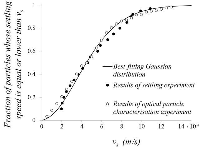
FIGURE 19. Distribution of settling speeds in the mixture of particles used in the experiments.
