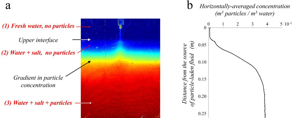
FIGURE 10. Steady-state distribution of particles in the tank in a typical experiment (experiment h, cf. table 2). Image a) illustrates the steady-state concentration of particles in the tank using false colours; image b) shows the horizontally-averaged particle concentration profile.
