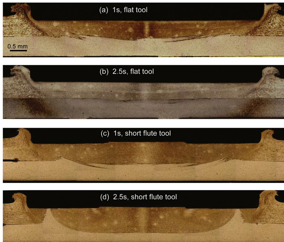
**Fig. 3.** Micrographs of sections through friction stir spot welds in dissimilar Al alloys in the horizontal lap configuration (all welds made at 2000 rpm, with 0.2 mm plunge): (a,b) flat tool, for dwell times of 1 s and 2.5 s respectively; (c,d) short flute tool, again for 1 s and 2.5 s respectively.
