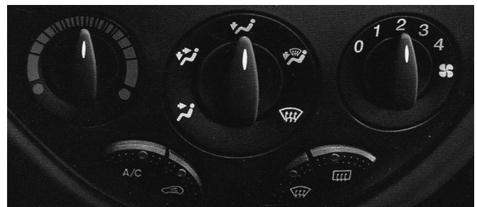
Fig. 3. Heating controls for the 1999 Ford Focus, where the centre knob for distribution control is larger than the knobs either side of it. Image source: Malcolm (1998).
