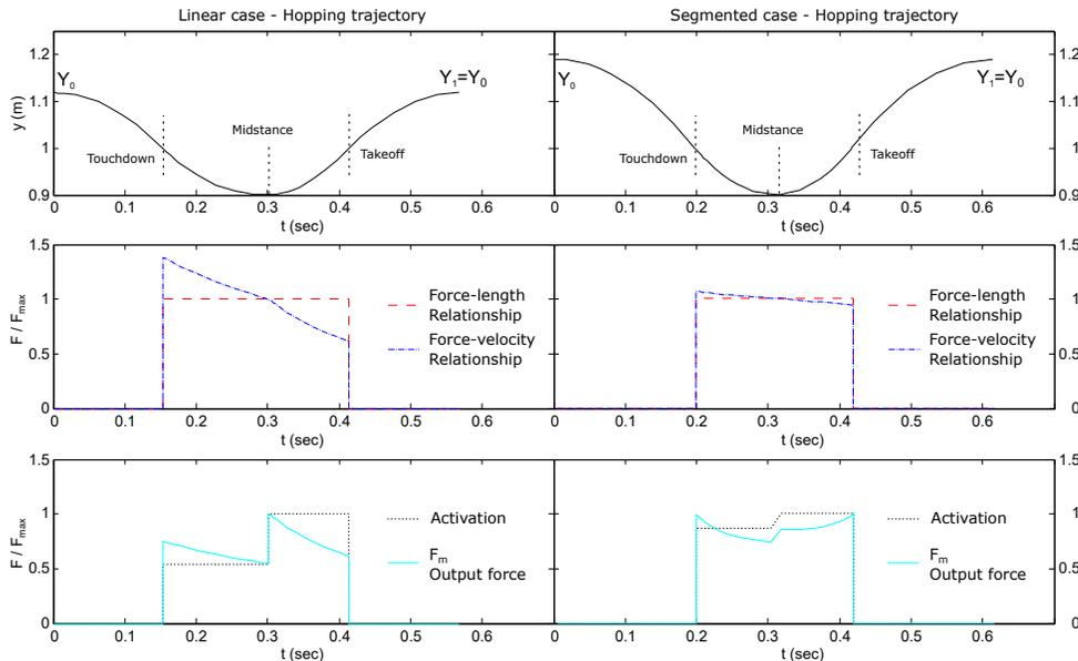
**Figure 3.** Example of the combined influence of force-length, force-velocity and activation upon the maximum force, resulting in the output force. The adopted force-length was of constant behavior, while the force-velocity was of linear behavior. The activation pattern is smaller until mid-stance, and maximum after it to ensure maximal hopping height.
