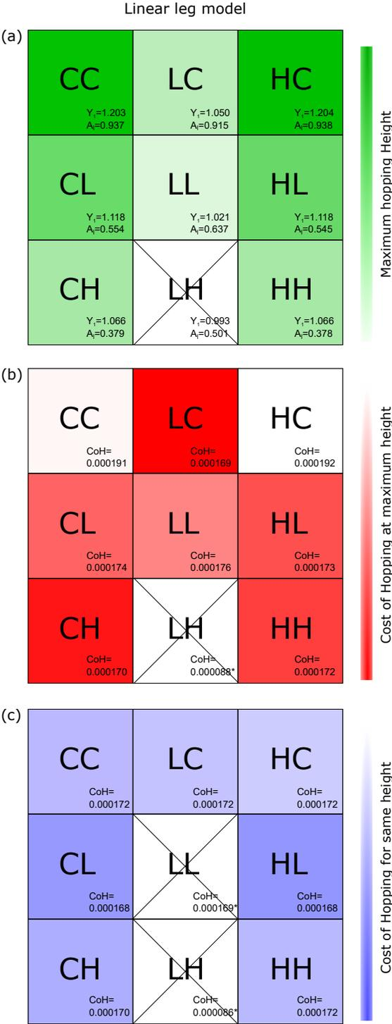
**Figure 4.** Results for the Linear Model. Darker colors indicate good results, while the worst results are in white. While xC cases excel at hopping height, xH cases demonstrate a better energy efficiency at maximum hopping height. All cases behaved similarly at the same hopping height.  $A_l$  indicates the activation during landing, while  $y_1$  is the final hopping height, where  $y_0 = y_1$  (stable). Same height experiments adopted  $y_0 = 1.066$ .
