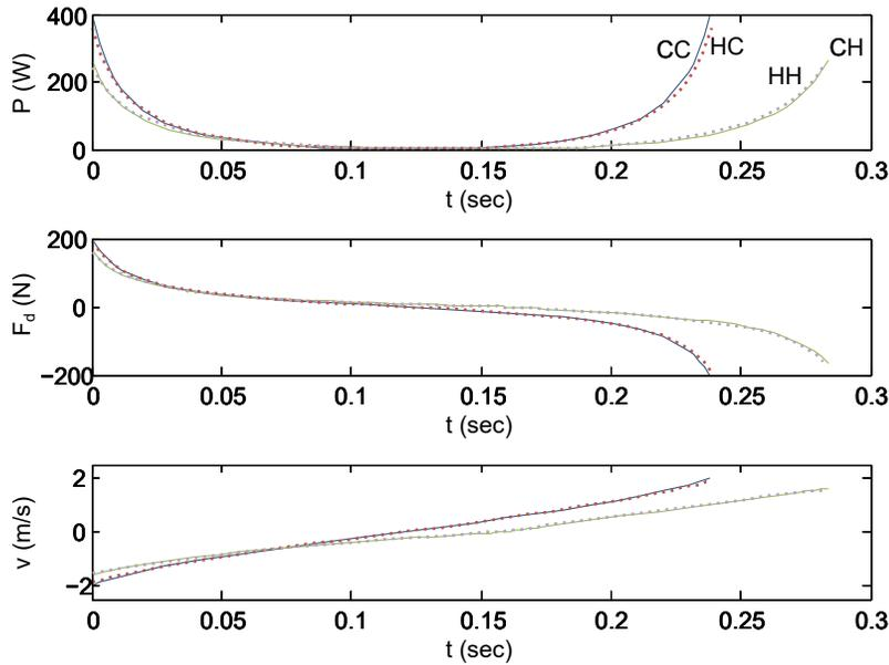
**Figure 7.** Comparison among the four cases. It is clear that the cases CC and HC require more power for a shorter period, while the cases HH and CH waste less power for longer periods. HH uses approximately the same amount of power that CH uses, but for a shorter period during maximum hopping.
