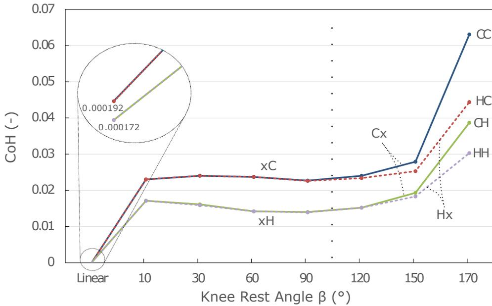
**Figure 6.** Different values for  $\beta$  result in different energy efficiencies for the cases xC and xH. As the knee resting angle increases ( $\beta > 90^\circ$ ) the differences between Cx and Hx can also be seen. The condition  $l_0 = 1$  was kept for all experiments, and the link geometries obeyed the Eq. (8).
