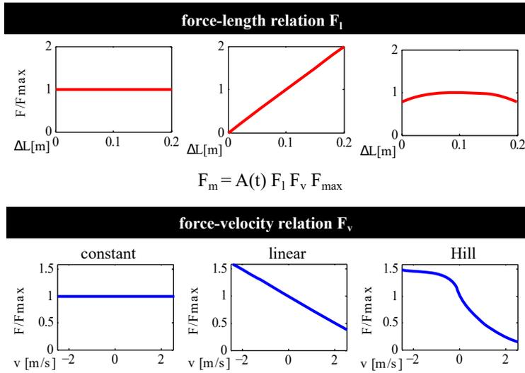
**Figure 2.** Pictogram with three force-length and three force-velocity relations. As the muscle is activated differences in length and velocity affect the force output from the model, and the Hill-type model is the model that most closely resemble the behavior of a biological muscle. This figure is adapted from Haeufle et al. 2010 [8].
