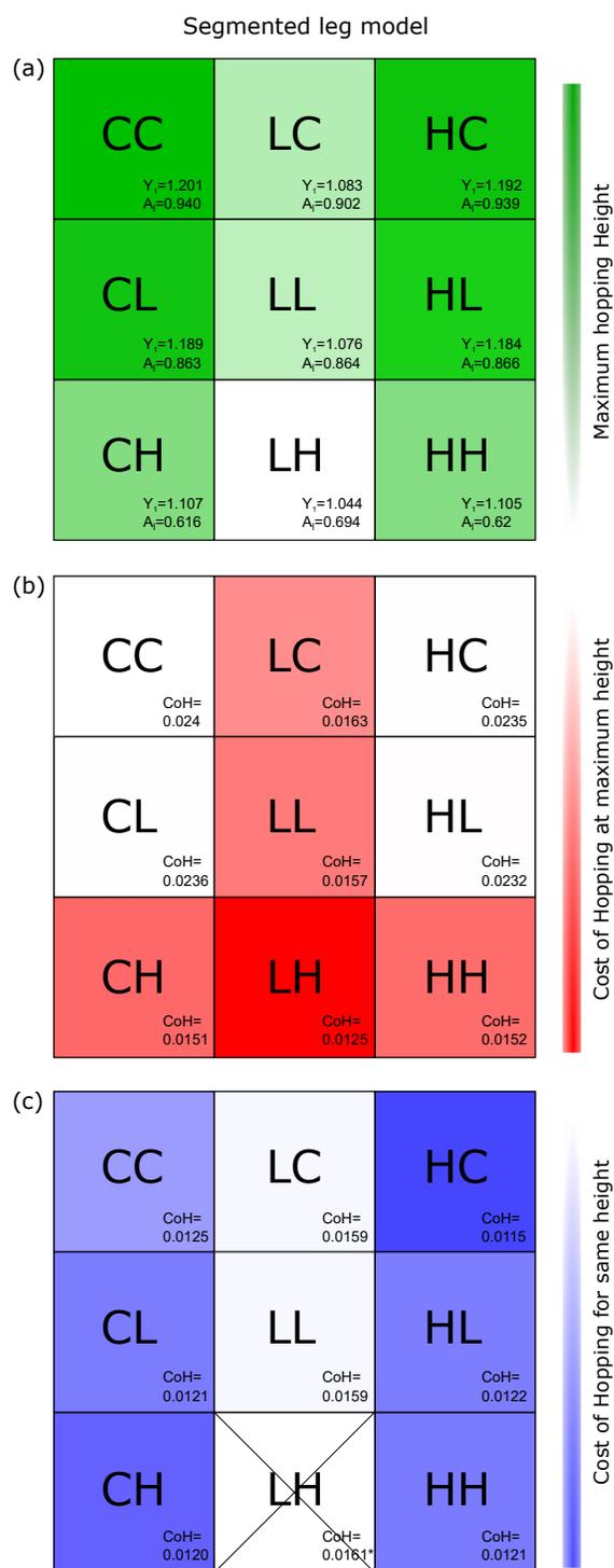
**Figure 5.** Results for the Segmented Model. Darker colors indicate good results, while the worst results are in white. Unlike the previous results, xC cases excelled at the hopping height criteria. As with the Linear Model, the xH cases are the most energy efficient at maximum hopping height, while Cx and Hx cases excel when hopping at the same height. Same height experiments adopted  $y_0 = 1.075$ .
