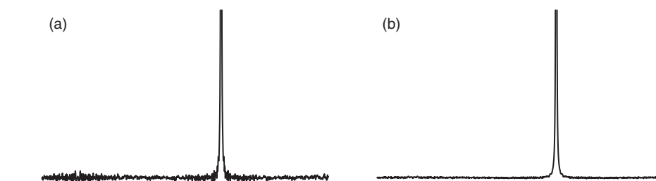
Fig. 5.6 Spectrum (a) is from an FID which has been digitized using a 6 bit ADC (i.e. 64 levels); the vertical scale has been expanded 10 fold so that the digitization sidebands are clearly visible. Spectrum (b) is from an FID which has been digitized using an 8 bit ADC (256 levels); the improvement over (a) is evident.
