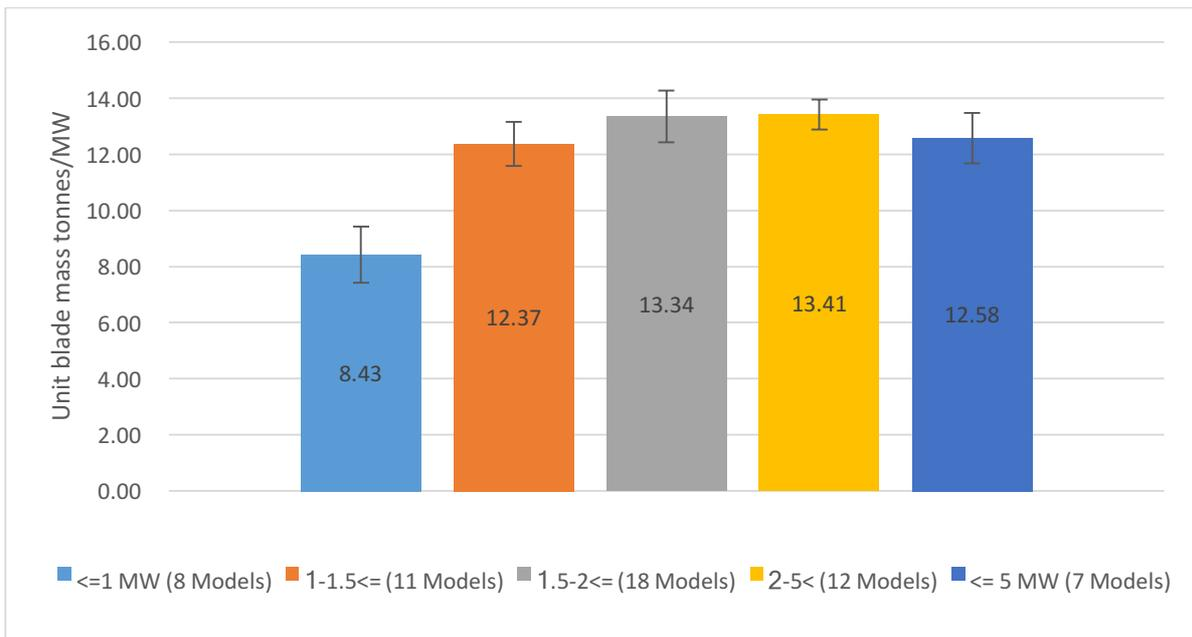
Figure 3: Blade mass per unit rated power for the different turbine size classes.
