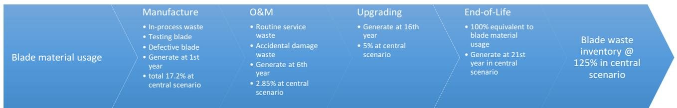
Figure 8: Waste generation flow from manufacture to end-of-life.
