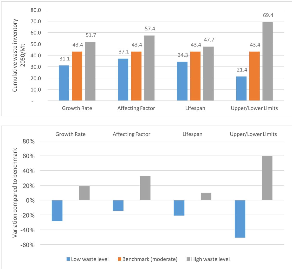
Figure 9 Upper: Global wind turbine blade waste 2050 in million tonnes (Mt), showing the effect of three different projection scenarios for each of three governing factors. "Affecting factor" includes waste contributing factors during both manufacture and O&M. The final column shows the maximum and minimum waste values obtained by combining the factors. Lower: Waste variation compared to benchmark in %.
