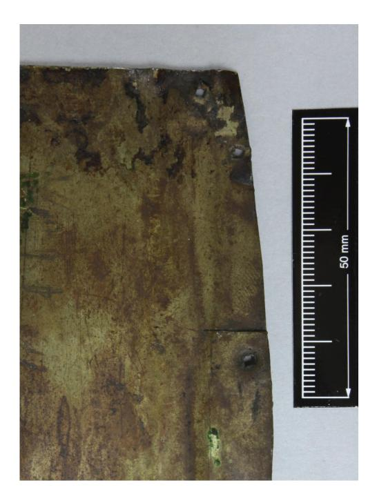
Fig. 3. Detail showing the square nail holes in the Forbes fragment. Scott Polar Research Institute, University of Cambridge, with permission.
