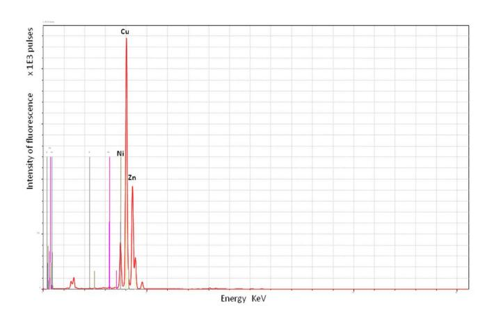
Fig.4. Graph showing results of qualitative analysis of the Forbes fragment by pXRF.
