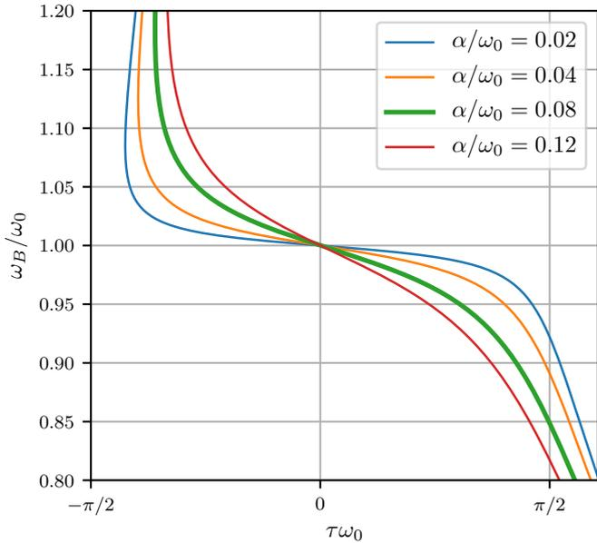
Figure A.1: Curves (A.6) for different values of the nondimensional damping  $\alpha/\omega$ , zoomed in to the approximate range for  $\omega$  for thermoacoustic applications fixed to  $\omega_0 \pm 20\%$ . In the following we use  $\alpha/\omega = 0.08$ .
