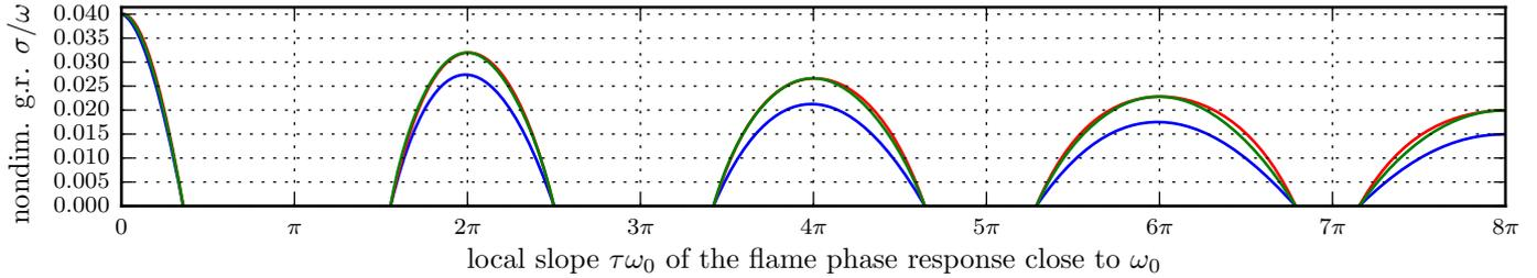
Figure 8: Linear growth rates (g.r.) of: the original equations of the system (2.3) with delay (blue), the truncated equations of the method of averaging (red), the equations of the method of multiple scales (green). These results are for  $\beta/\alpha = 2$ ,  $\alpha/\omega = 0.08$ .
