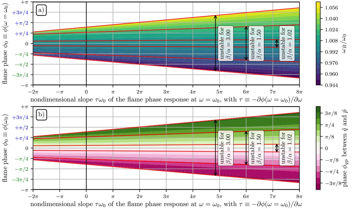
Figure 6: Same as Fig. 5, but for a level of acoustic damping  $\alpha/\omega_0 = 0.04$  instead of 0.08. Since the investigated range of  $\beta/\alpha$  is the same as Fig. 5, this presents smaller forcing terms  $f$  on the right hand side of (18), the acoustic field is less perturbed and the thermoacoustic frequency  $\omega_B$  in a) is closer to  $\omega_0$  than in Fig. 5.
