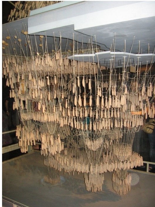
302 Figure 10-Recreation of Gaudi's hanging model for the Sagrada Familia, Barcelona. Photo reproduced 303 under CC-BY-SA/© Canaan [93].
