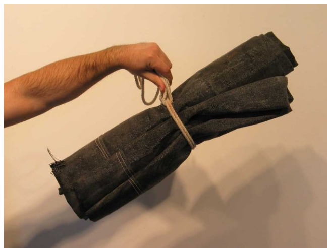
Figure 18 – Easily transportable flexible formwork. Photo: Mark West (C.A.S.T.).
